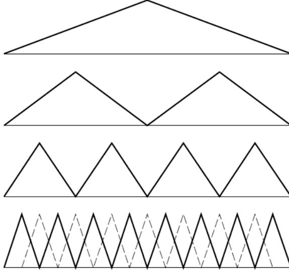
Figure 5.3: Piecewise linear hierarchical basis (solid line) and nodal point basis (dashed line) [32]
