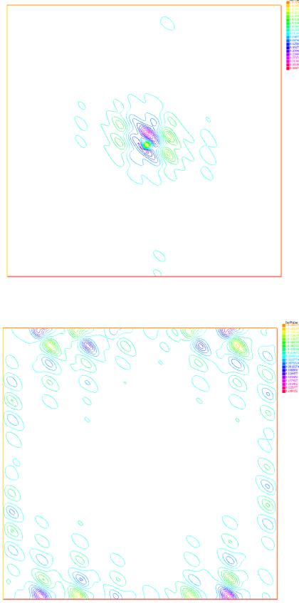
Figure 3.6: A true eigenfunction, localized close to the defect (top), and a “spurious” eigenfunction, localized close to the boundary (bottom).
