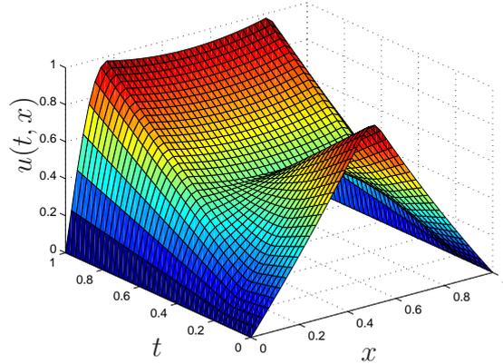
Figure 6.4: Altitude of the rope as a function of  $t$  and  $x$ .
