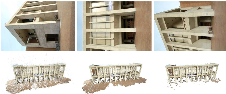
Figure 7.11: Hall data-set. Top: 3 among 61 input images. Bottom: from left to right: our point cloud, the PMVS point cloud found in the package, the PMVS point cloud which we obtain.
