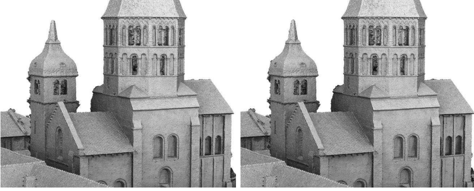
Figure 7.3: Cluny-26-Big refined mesh with memory threshold th = 1GB and th = 512MB . There is almost no difference in 2 meshes.
