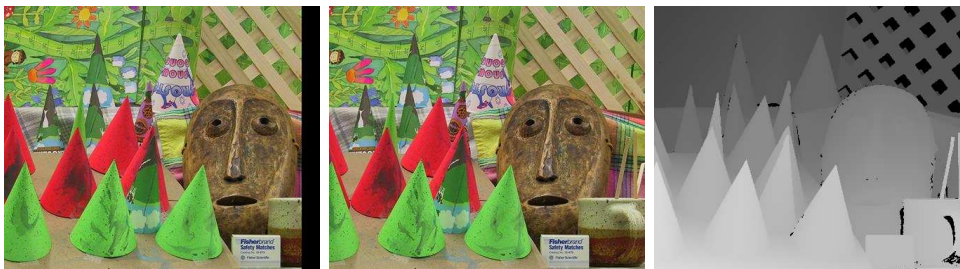
Figure 2.4: Disparity of rectified images. The third image displays the disparity measure of the second image with the first one.
