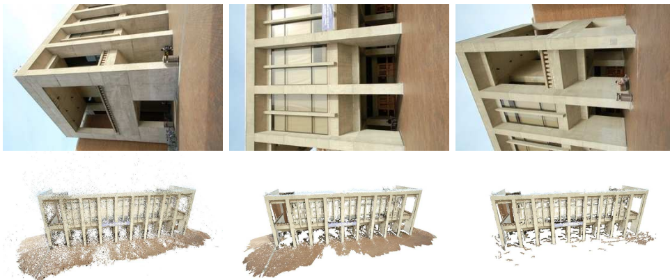
Figure 7.11: Hall data-set. Top: 3 among 61 input images. Bottom: from left to right: our point cloud, the PMVS point cloud found in the package, the PMVS point cloud which we obtain.
