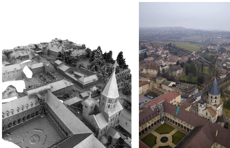
Figure 4.11: Results on Cluny data-set. Cluny Abbey built from 30 images taken from a balloon (© B.Vallet/IMAGINE) and an image of data-set.
