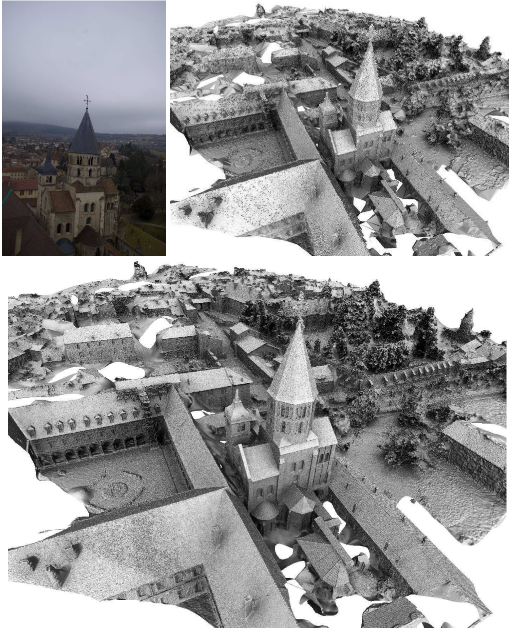
Figure 7.2: Cluny-26-Big datasets with 26 images of 56 MPixel. Left: initial mesh. Right: final mesh in the full resolution with th = 1GB .
