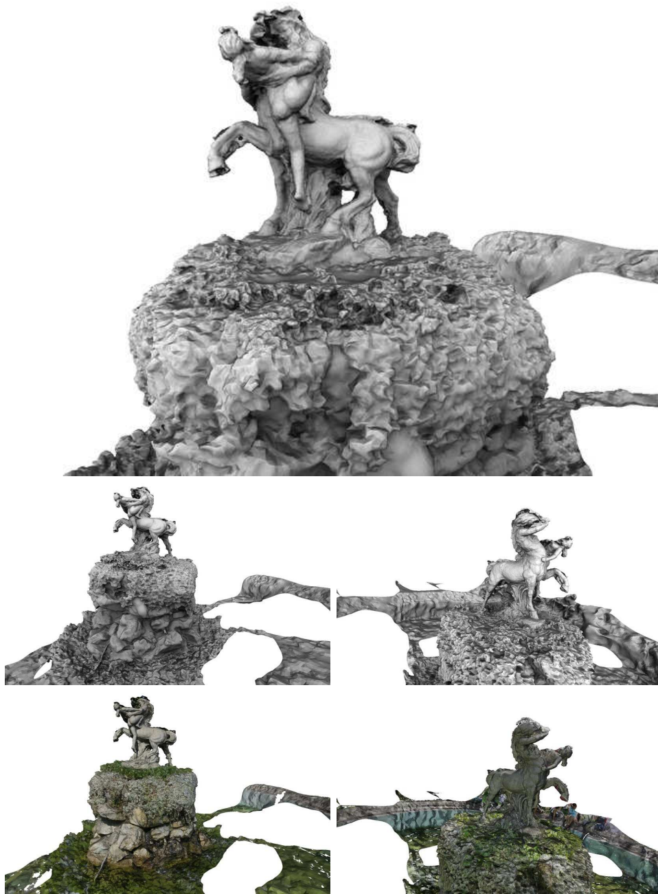
Figure B.3: Result of Detenice data-set with demi-resolution (mipmap 1: 750K Pixel). The result with full resolution does not improve the quality of the mesh. It might be due to the limited image quality (chromatic aberration, blur, etc) which leads to not accurate calibration and multi-view stereo. Last 2 images show the mesh with texture.
