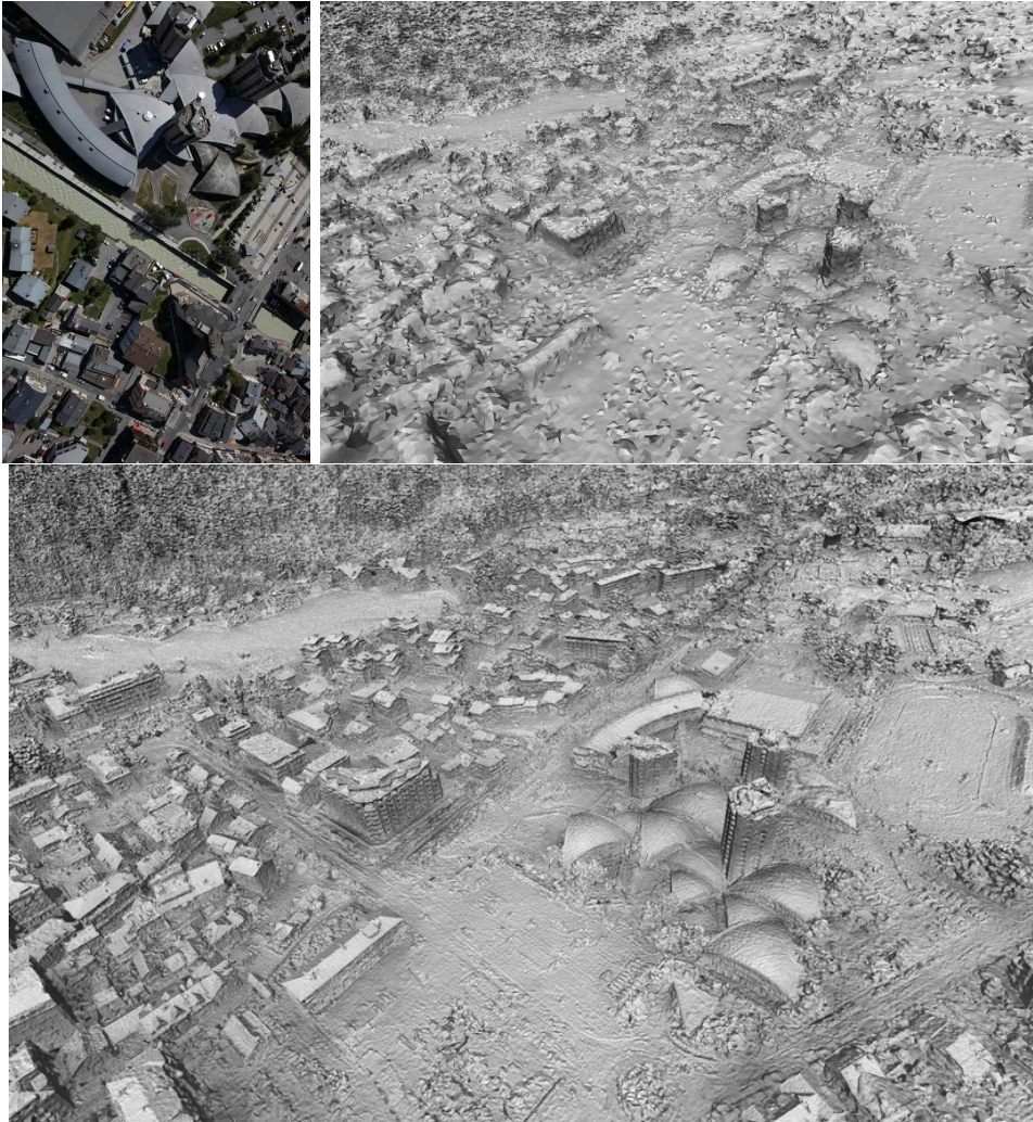
Figure 7.8: Chamonix (1595 images of 5.3 MPixels): initial mesh ( 747 K facets) and final refined mesh (36.3 M facets).
