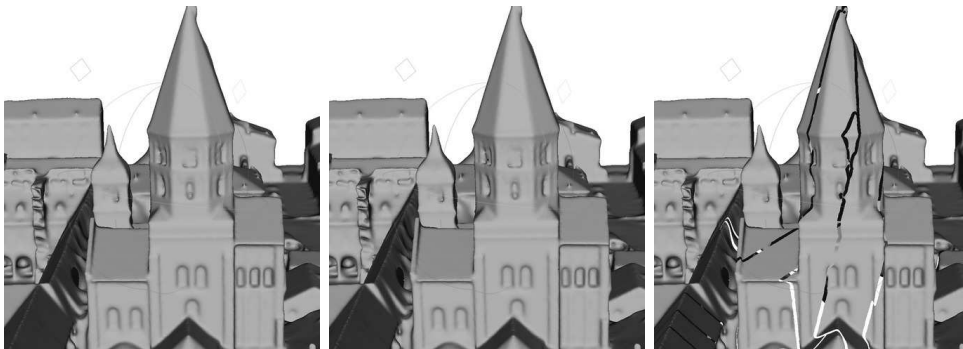
Figure 7.6: Cluny-26-Big: (Level 1) refined meshes are smoothed with 30 Laplacian operations. Left to right: mesh with serial refinement, mesh is merged from 8 partial refined sub-meshes, union of these 8 refined sub-meshes. There is visually no crack in merged mesh, which prove the success of the merging algorithm.
