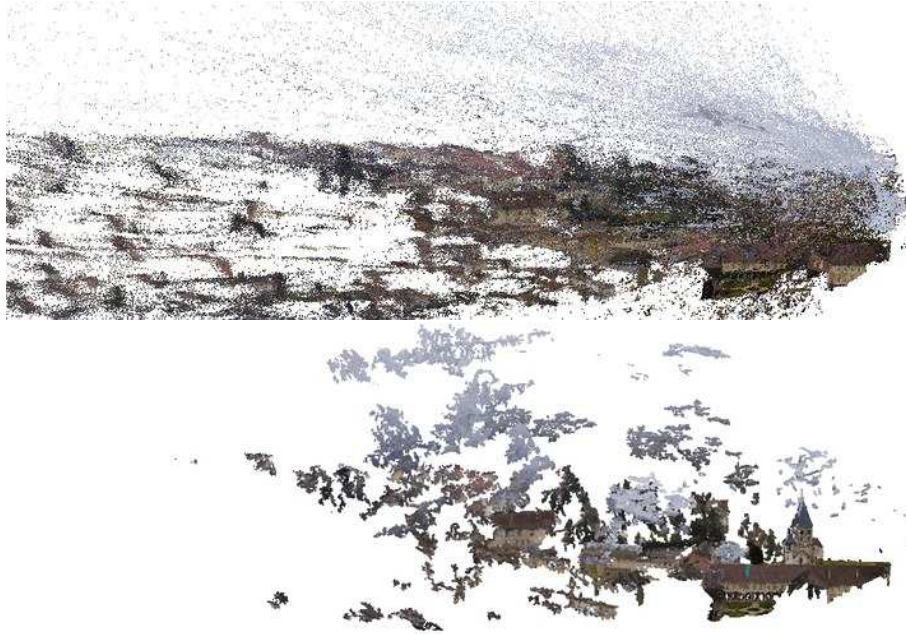
Figure 7.9: Point cloud generated by our GPU sweeping-plane method (up) and PVMS2 (bottom). PMVS point cloud has less noise but also less complete.
