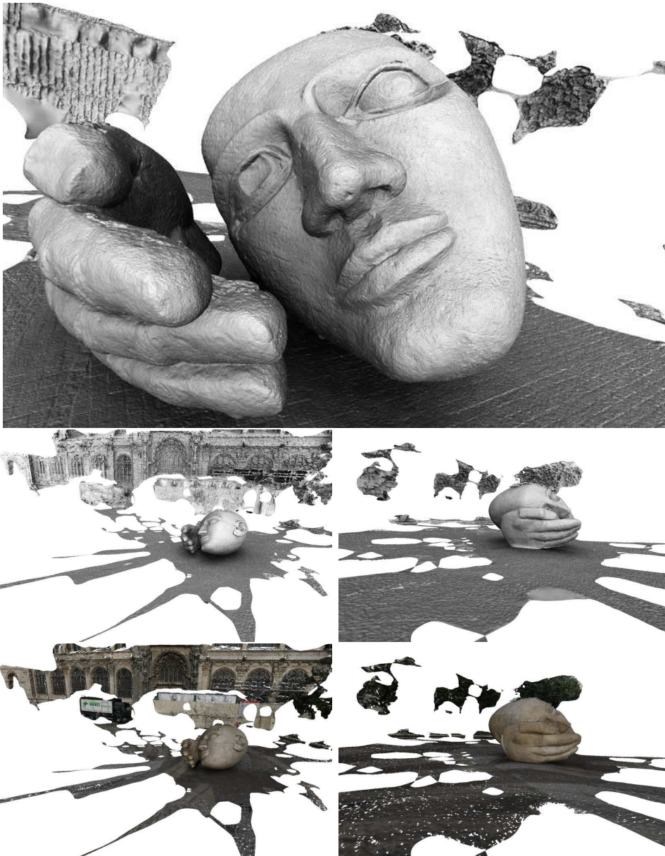
Figure B.2: Result of Head data-set with full resolution (mipmap 0: 6 MPixel). This data-set is very well calibrated, so that the reconstructed mesh is highly accurate. Last 2 images show the mesh with texture.
