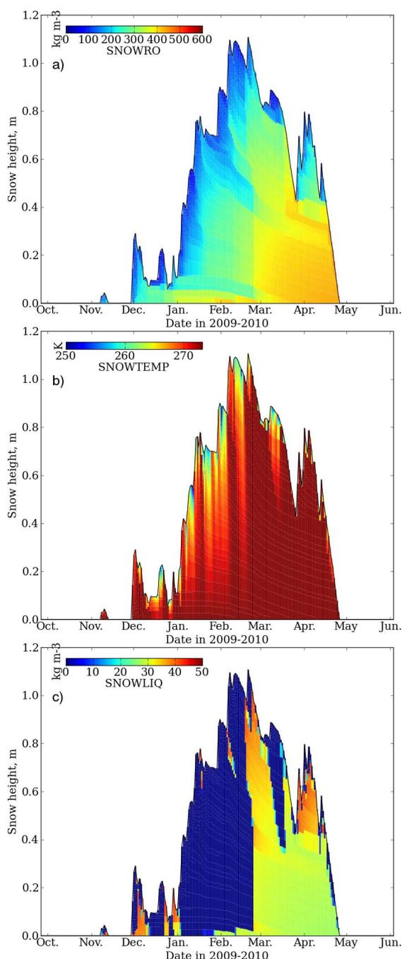
**Fig. 5.** Example of visualization of the time series of snowpack profile properties simulated by the snowpack scheme Crocus in SURFEX. The simulation used is the year 2009–2010 of simulation from the model run carried out at Col de Porte, France (see Sect. 5.1 for details). The data represented here are (a) snow density ( $\text{kg m}^{-3}$ ), (b) snow temperature (K), and (c) snow liquid water content ( $\text{kg m}^{-3}$ ).
