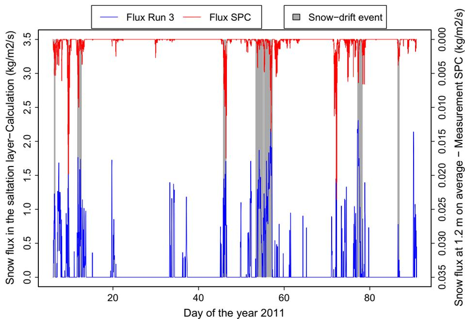
**Fig. 12.** Snow particle fluxes in  $\text{kg m}^{-2}\text{s}^{-1}$ : measured by SPC at 1.2 m on average above the snow surface (red) and simulated by the model in the saltation layer using Sørensen's formulation (Run 3, blue). Blowing snow events from the 10-year database are shown in gray. (For interpretation of the references to colour in this figure legend, the reader is referred to the web version of this article.)
