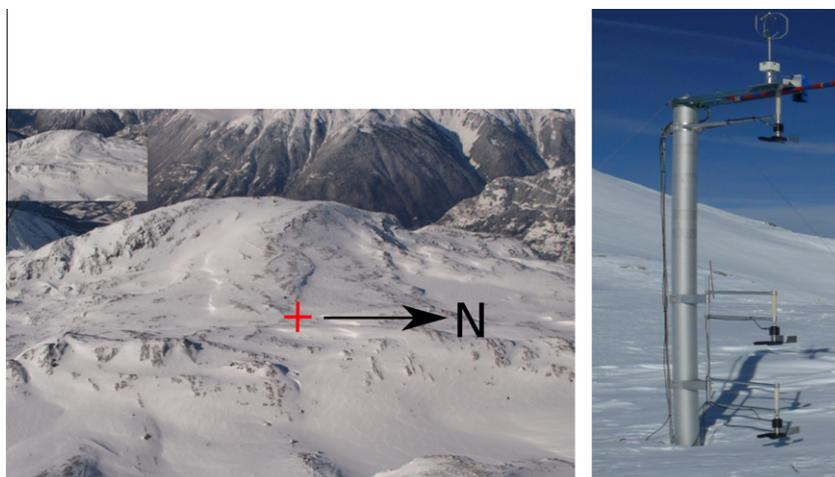
**Fig. 1.** Left: view of the experimental site. The red cross indicates the location of the northern AWS. Right: experimental set-up for measuring snow flux profiles at Col du Lac Blanc during winter season 2010–2011. (For interpretation of the references to colour in this figure legend, the reader is referred to the web version of this article.)
