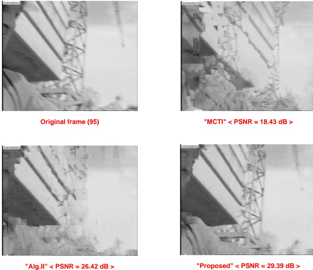
Figure 4.13: Visual result comparisons among the original frame (top-left), the SI estimated by the MCTI technique (top-right), the final SI estimated by Alg. II (bottom-left), and the final SI estimated by the proposed method (bottom-right), for frame number 95 of Foreman sequence, for a GOP size of 8 ( $QI = 8$ ).
