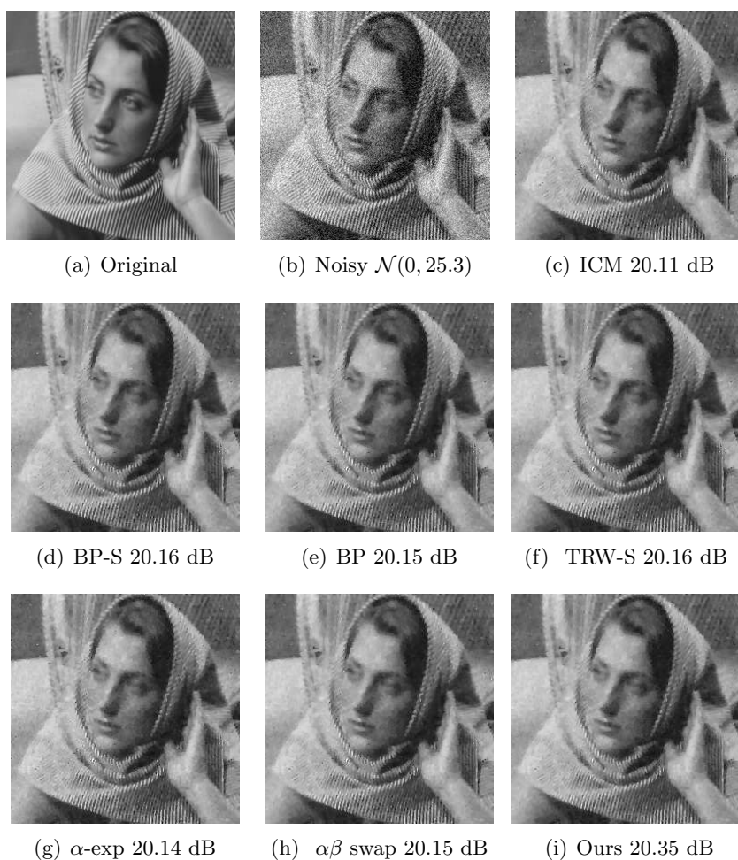
Figure 6.3: The image restoration results for truncated \ell_1 - \ell_2 prior with threshold T = 50 , \ell_2 data fidelity term, and \lambda = 2 .
