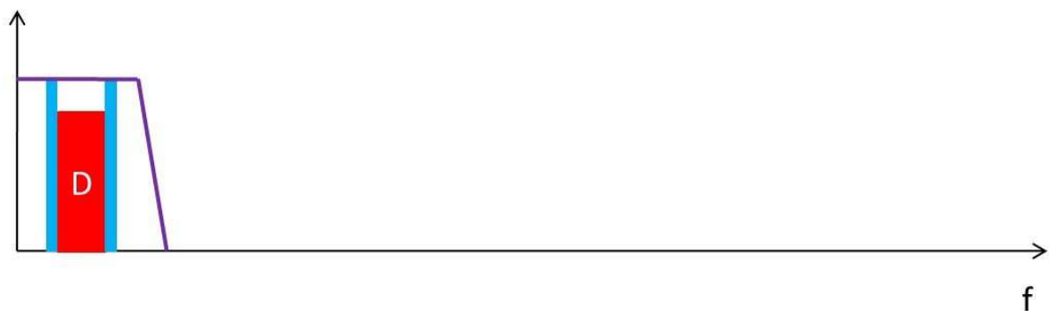
Fig.1. 13 - Wanted channel after mixing and LPF
