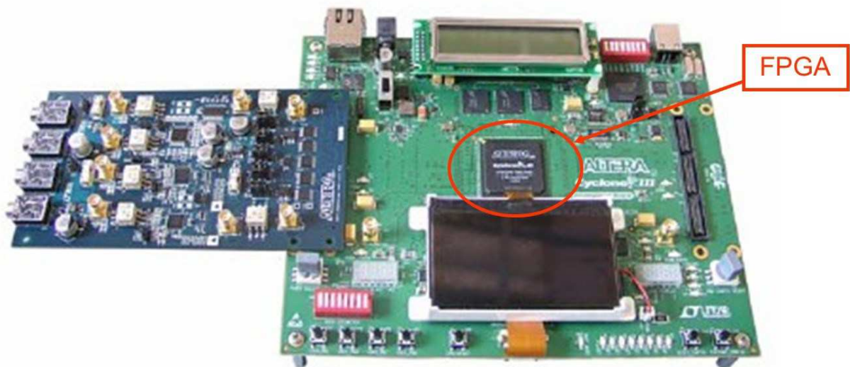
Fig.4. 14 - Board HMSC with stratix III
