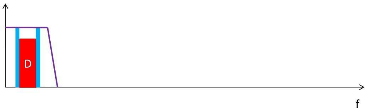
Fig.1. 13 - Wanted channel after mixing and LPF
