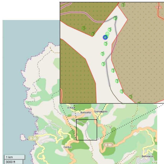
Figure 2.19: Map of the Ersá wind farm. The zoomed portion of the map shows the positioning of the 13 turbines (highlighted by green circles) situated along the crest of Torricella. The blue circle shows where the measuring mast was positioned during the experiment. The exact coordinates of the mast are 42°58.153'N by 9°22.809'E
