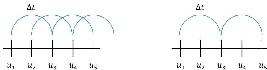
Figure B.1: Illustrative diagram of the two different methods for obtaining the differences of the velocity.
