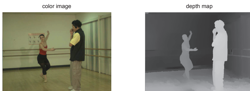
Figure 2.13: In MVD, at each instant the output of each camera is the color image and the corresponding 8-bit depth map.
