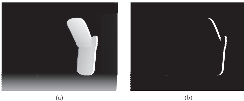
Figure 5.16: The estimated left depth (a) and the estimation of occluded regions \widehat{O}_L (b)
