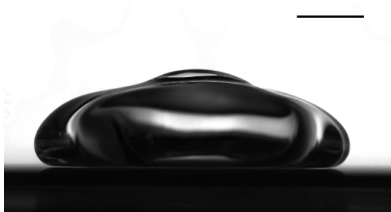
Figure I.20 – Side view of a Leidenfrost drop puddle deformed by a chimney instability. Vapor underneath is less dense than liquid on top. As the interface is deformable, buoyancy effects make the vapor try to escape upwards and form a dome before bursting. Scale shows 5 mm.
