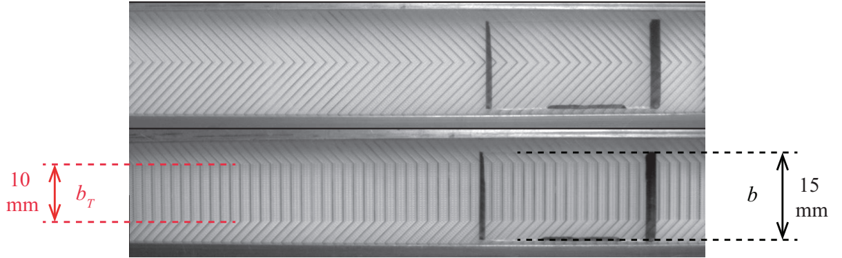
Figure III.9 – Comparison between two textures entraining a glass slider of length a = 30 mm, width b = 15 mm and thickness c = 1 mm (resulting in a weight M around 1 mg). Top texture is the “classical” herringbone. Bottom one corresponds to the “truncated” herringbone, which has a central straight section of length b_T (fixed to 10 mm) perpendicular to motion, hence having a null viscous propelling contribution.
