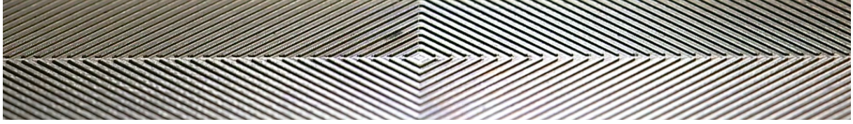
Figure II.27 – View of the texture resulting from joining two herringbones of opposite polarization and facing each other: we see concentric squares whose diagonals are the axis of symmetry of the herringbones.
