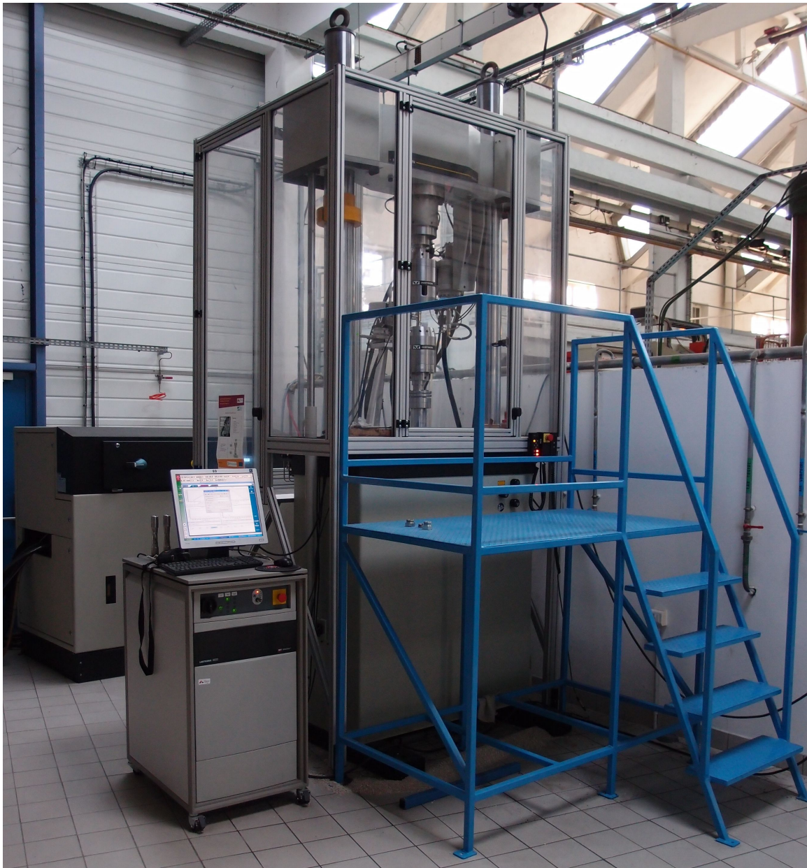
FIGURE III.1 – Machine d'essai de fatigue servo-hydraulique multi-axiale Instron 8850.
