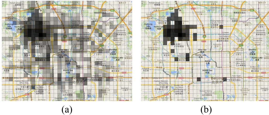
Figure 6.2: (a) Division of the map of Beijing into regions of size 0.658 \times 0.712 km. The density of each region represents its “score”, that is, how frequently users visit it. (b) The 50 selected regions. These regions are the ones with highest density between the whole set of regions.
