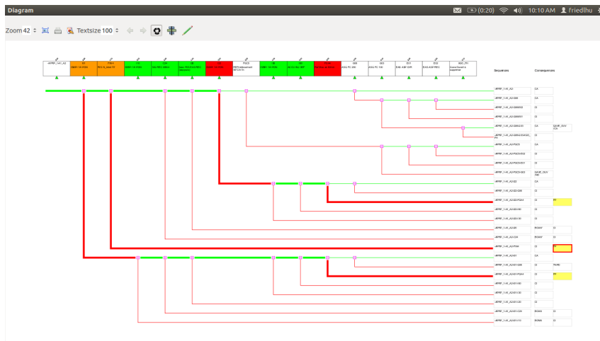
Figure 8.18. Color inking in event trees I: The mitigation respective a certain consequence is inked in colors.
