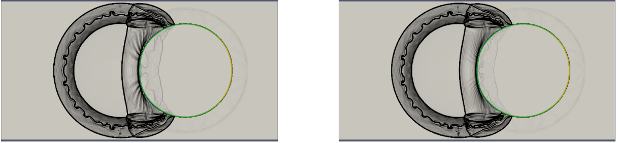
Fig. 3.16: Gradient density field in the fluid and normal stress distribution in the cylinder at time 4.7 \times 10^{-3} s for 100 solid particles (left) and 200 solid particles (right).
