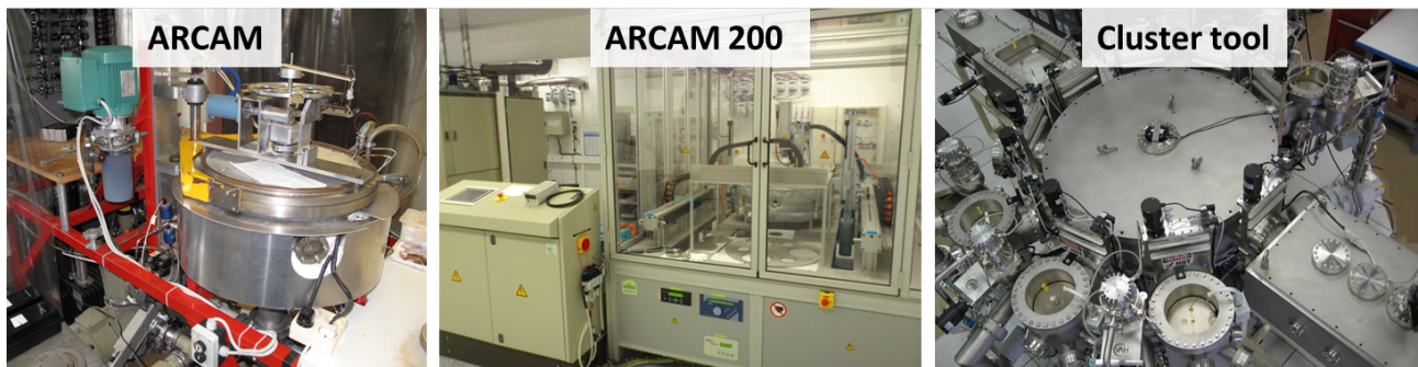
Fig. 2.1 – Pictures of some PECVD reactors: ARCAM the 30 years old home-built reactor 3 , ARCAM 200, the automated reactor installed in Thales TRT clean room and the Total/LPICM cluster tool.
