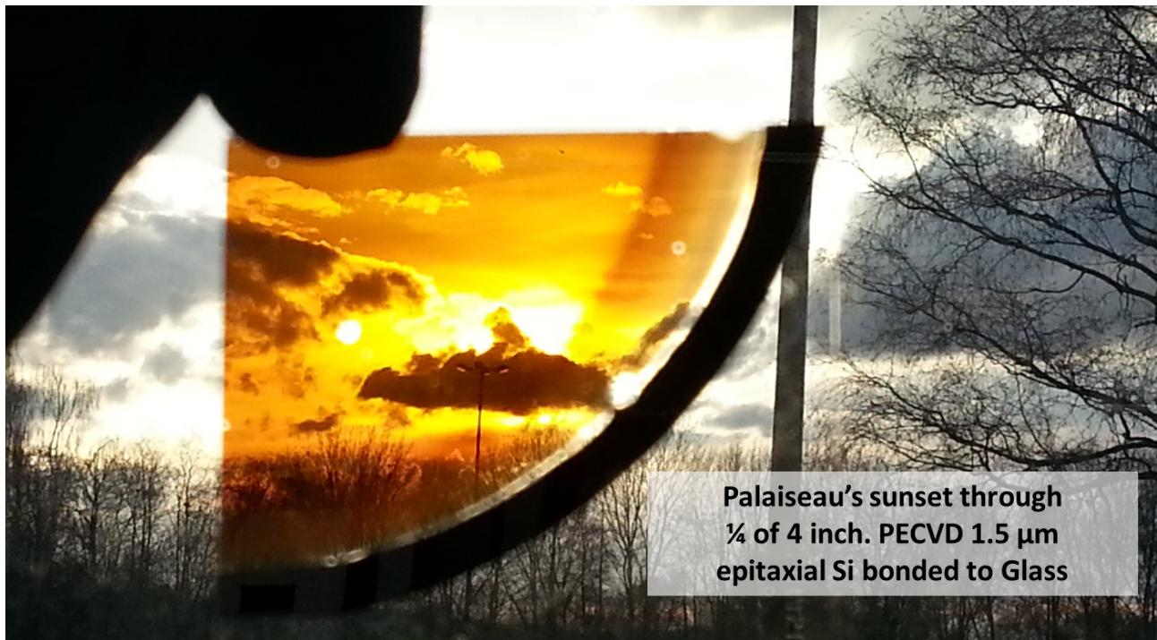
Fig. 4.29 – Experimental proof of transmission losses in 1.5 \mu\text{m} thick epitaxial silicon bonded to glass substrate.
