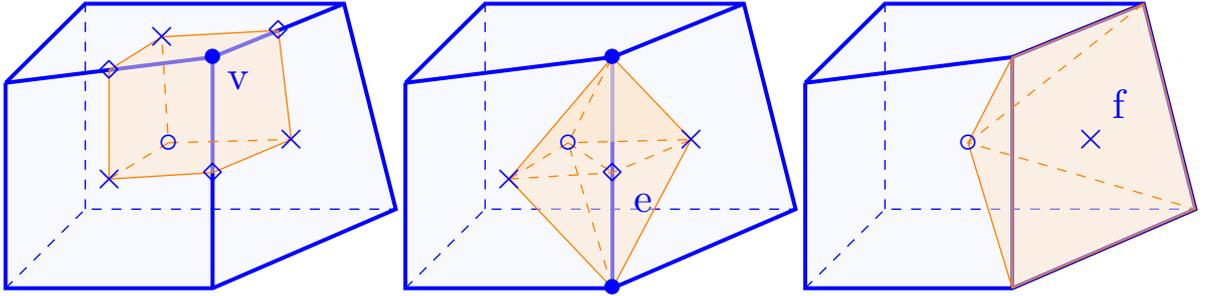
Figure 7.5 – Example of partition of a hexahedral cell  $c$ . Left:  $\mathbf{p}_{v,c}$  for a vertex  $v \in \mathcal{V}_c$ ; Middle:  $\mathbf{p}_{e,c}$  for an edge  $e \in \mathcal{E}_c$ ; Right:  $\mathbf{p}_{f,c}$  for a face  $f \in \mathcal{F}_c$ . Crosses indicate barycenters of faces and diamonds barycenters of edges.
