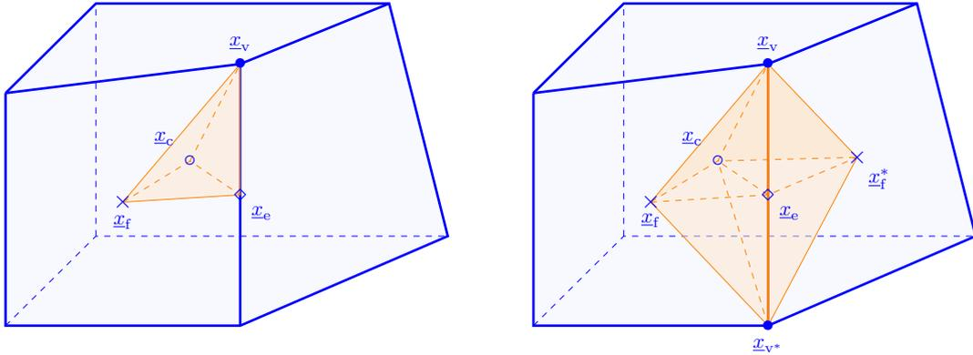
Figure 5.1 – Left: Elementary subsimplex  $\mathfrak{s}_{v,e,f,c}$ ; Right: The four elementary subsimplices ( $\mathfrak{s}_{v,e,f,c}$ ,  $\mathfrak{s}_{v,e,f^*,c}$ ,  $\mathfrak{s}_{v^*,e,f,c}$ ,  $\mathfrak{s}_{v^*,e,f^*,c}$ ) associated to an edge  $e \in E_c$ .
