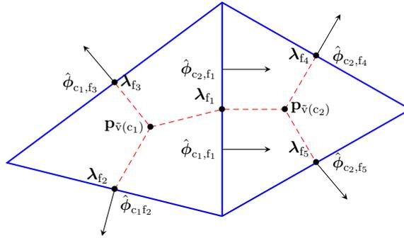
Figure 8.4 – Positioning of DoFs within the hybrid formulation.
