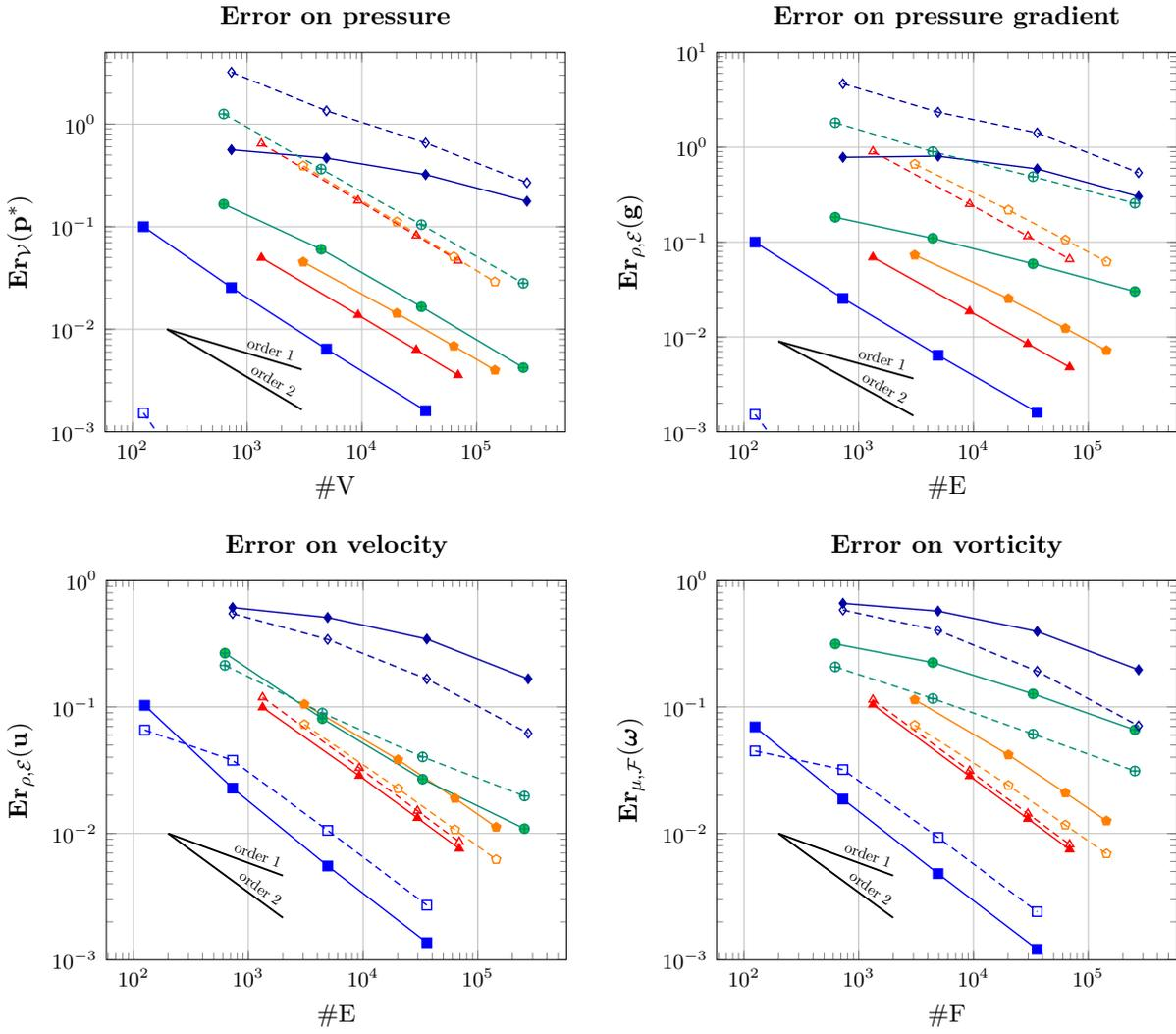
Figure B.5 – Discrete error on the pressure (upper left), on the pressure gradient (upper right), on the velocity (lower left), and on the vorticity (lower right) for the vertex-based pressure scheme using the SUSHI-like reconstruction operators. Essential BCs are considered: EDL with labels A and EPL with labels B.
