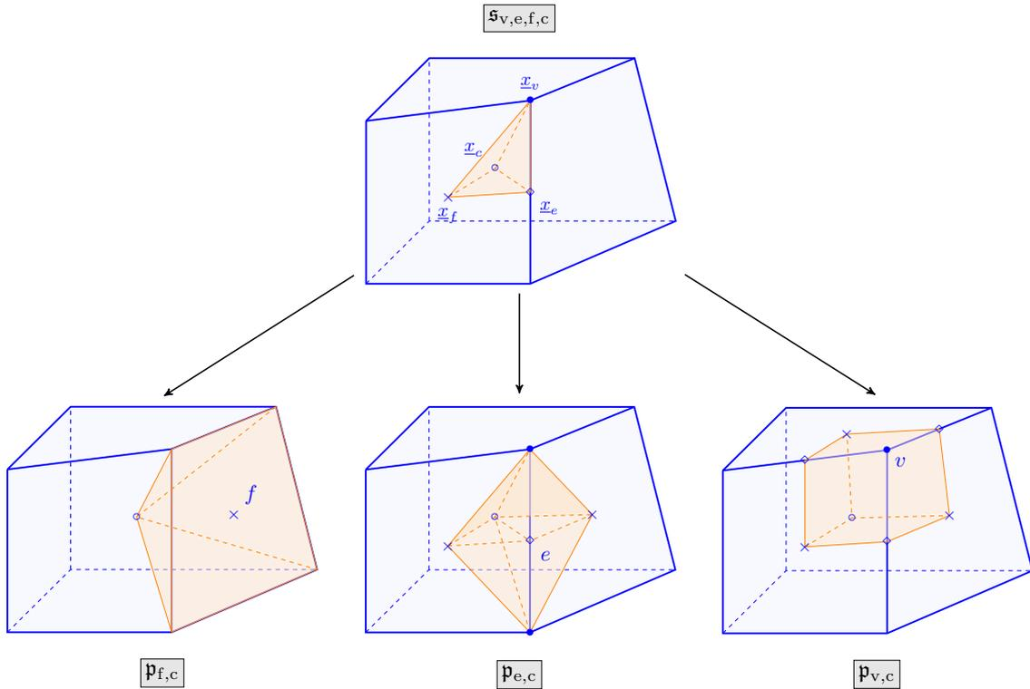
Figure 5.4 – Hexahedral mesh cell  $c$ . Above: Elementary subsimplex  $\mathbf{s}_{v,e,f,c}$  of the barycentric subdivision; Below: Example for  $\mathbf{p}_{f,c}$  (left),  $\mathbf{p}_{e,c}$  (center), and  $\mathbf{p}_{v,c}$  (right).
