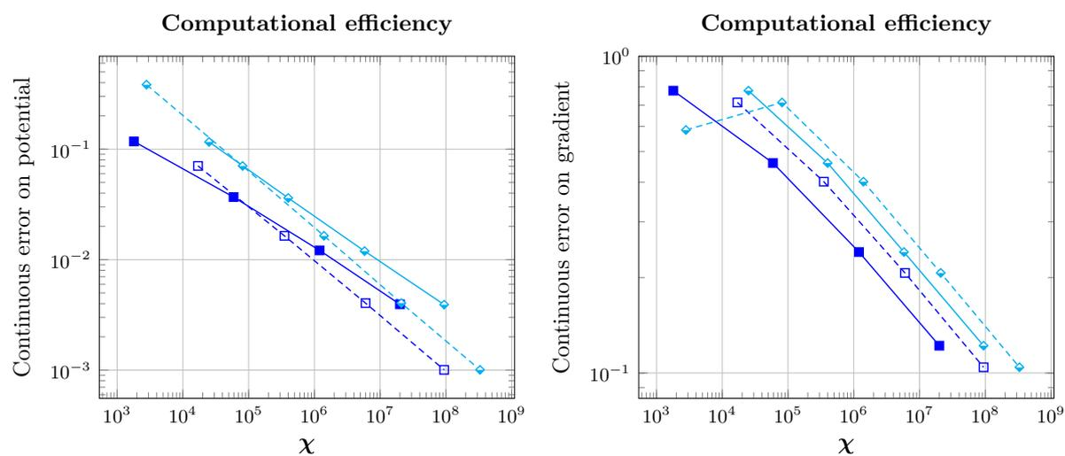
Figure 8.13 – Comparison of the cost-effectiveness between **Vb-SUSHI** (labels A) and **Hcb-SUSHI** (labels B) schemes for the error on potential in continuous norm (left) and the error on gradient (right) in continuous energy norm.
