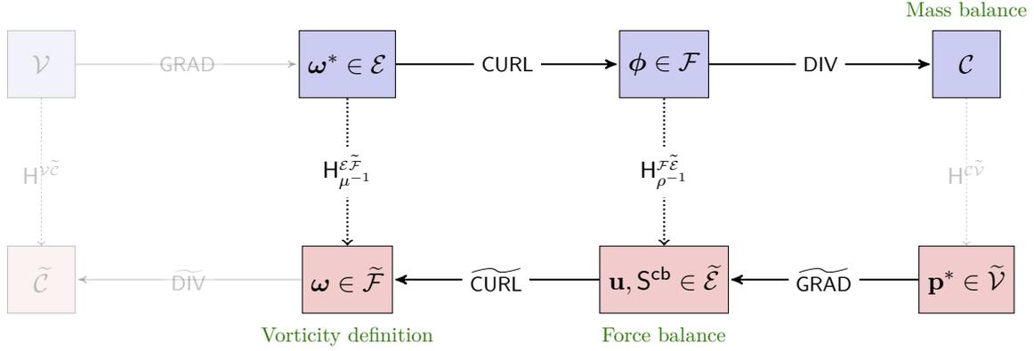
Figure 4.4 – Tonti diagram of cell-based pressure schemes for the Stokes equations.
