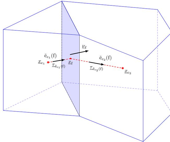
Figure 5.2 – Let  $c_1$  and  $c_2$  be two primal cells. For the face  $f \in F_{c_1} \cap F_{c_2}$ , we represent the dual edge  $\tilde{e}(f)$  (red dashed line) associated to  $f$ .  $\tilde{e}(f) = \tilde{e}_{c_1}(f) \cup \tilde{e}_{c_2}(f)$ .
