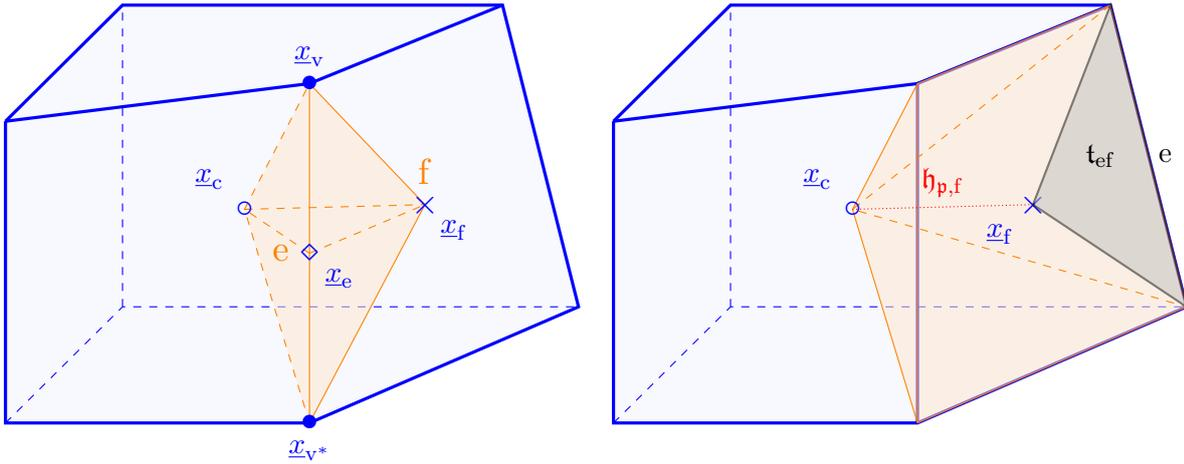
Figure 5.6 – Let  $c$  be a hexahedron. Left: For a face  $f \in F_c$  and an edge  $e \in E_f$ , the subvolume  $p_{ef,c}$  is highlighted. Right: For  $f \in F_c$ ,  $p_{f,c}$  (in orange), its height  $h_{p,f}$  (red dotted line), and the triangle  $t_{ef}$  (gray) for an edge  $e \in E_f$  are highlighted.
