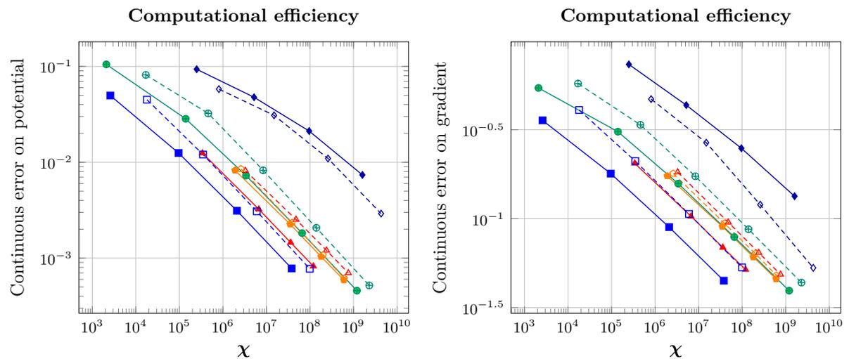
Figure 8.7 – Comparison of the cost-effectiveness between **Vb**-DGA (labels A) and **Hcb**-SUSHI (labels B) schemes for the continuous error on the potential (left) and the error on the gradient in continuous energy norm (right).
