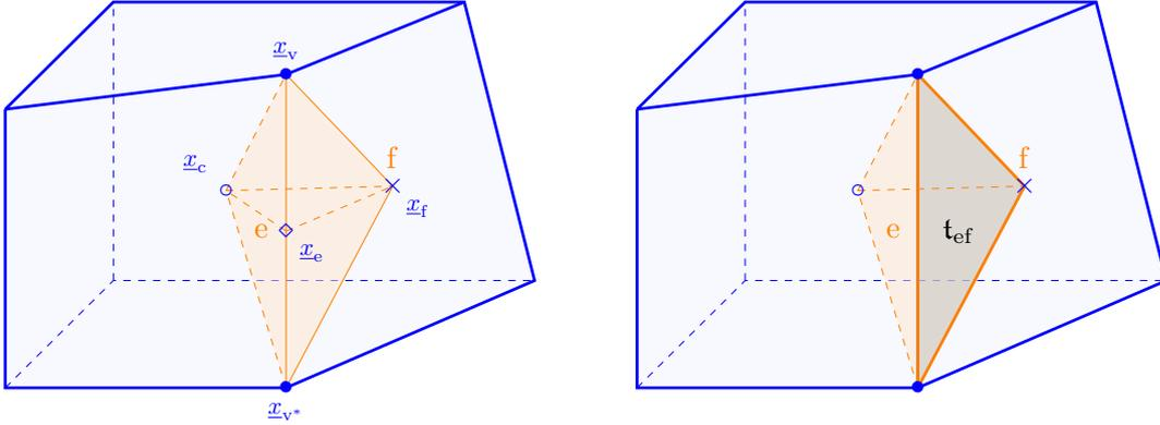
Figure 7.6 – Let  $c$  be a hexahedron. For a face  $f \in F_c$  and an edge  $e \in E_f$ , we highlight the subvolume  $\mathfrak{p}_{\text{ef},c}$  (left) and the triangle  $\mathfrak{t}_{\text{ef}}$  (right).
