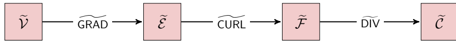
Figure 3.10 – Cochain complex induced by the discrete differential operator on the dual mesh.
