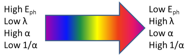
Figure 1-5 – Schematic representation of the evolution of the absorption depths as a function of the incident energy photon E_{ph} .
