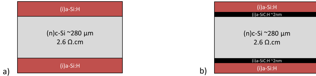
Figure 3-26 – Schematic representation of a passivated c-Si wafer with (right) and without (left) a thin a-SiC:H layer at the a-Si:H/c-Si interface.
