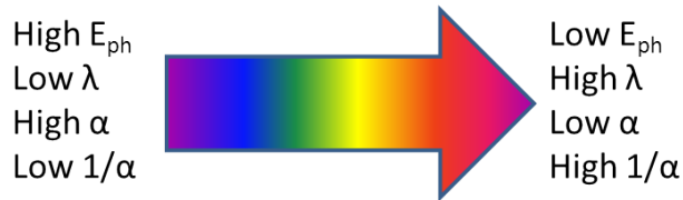
Figure 1-5 – Schematic representation of the evolution of the absorption depths as a function of the incident energy photon E_{ph} .
