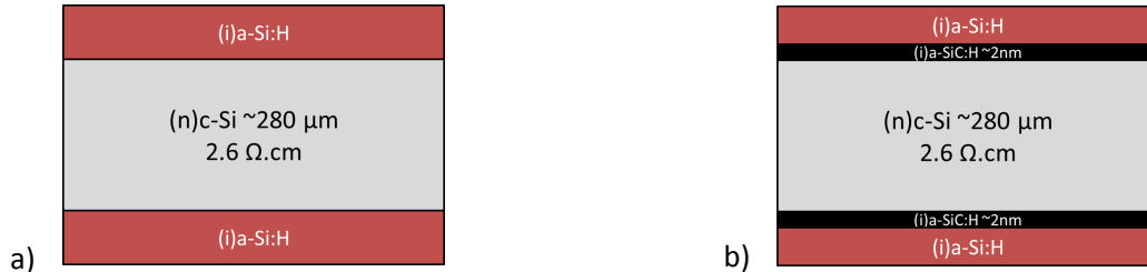
Figure 3-26 – Schematic representation of a passivated c-Si wafer with (right) and without (left) a thin a-SiC:H layer at the a-Si:H/c-Si interface.
