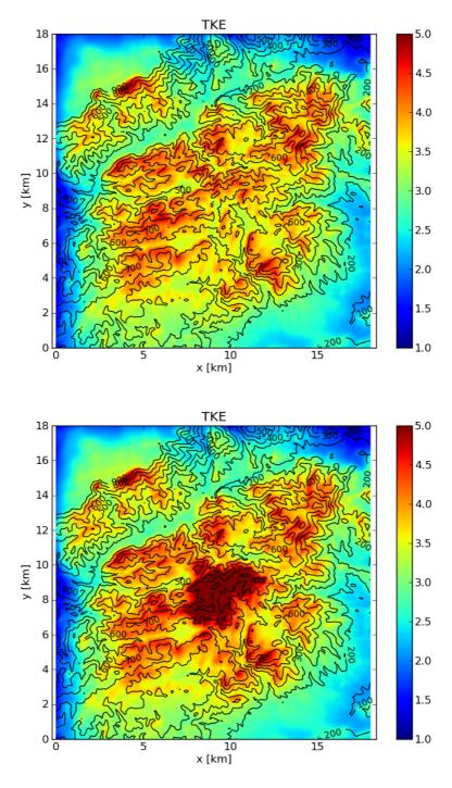
Figure 5.18: Annual average TKE at 80m above the ground a) CFD simulation without assimilation b) CFD simulation with assimilation
