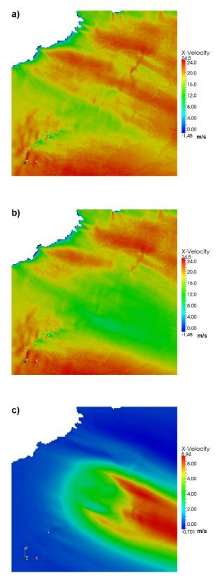
Figure 4.10: Velocity u component cross-section at 770 m altitude for a) CFD simulation without assimilation b) CFD simulation with assimilation c) difference between the CFD simulation without and with assimilation.
