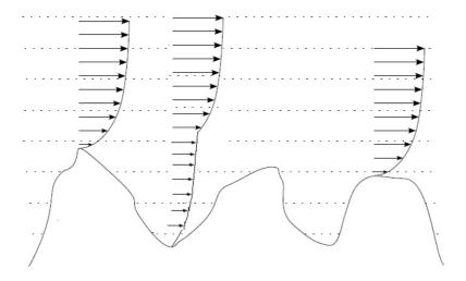
Figure 3.13: Extrapolation coupling method on complex terrain.
