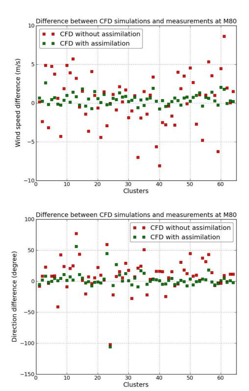
Figure 5.10: Difference between CFD simulations without assimilation and measurements, CFD simulations with cup assimilation and measurement and CFD simulations with sonic assimilation and measurement at M80 (80m) a) wind speed b) direction.
