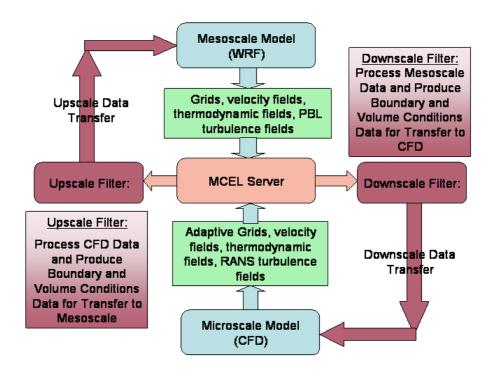
Figure 2.7: WRF-MCEL-CFD Coupling Conceptual: Initial model, Source: Coirier et al. (2007)
