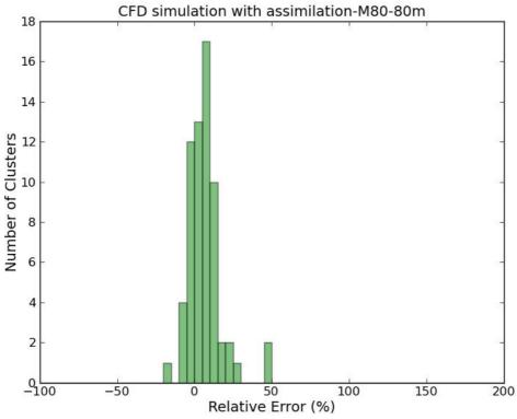
Figure 5.13: Wind speed relative error distribution for the 64 clusters at M80 (80m) location a) CFD simulations without assimilation b) CFD simulations with cup anemometers data assimilation.
