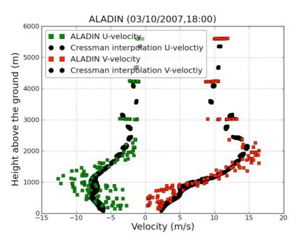
Figure 4.17: Imposed inflow along the north and west boundary using Cressman interpolation for  $r_L$ =8500 m and  $r_Z$ =100 m.
