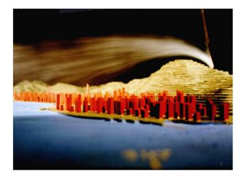
Figure 2.3: Flow separation on a model site for potential wind farm site (top) and Victoria Park on Hong Kong for wind structure at central in the boundary layer wind tunnel (bottom) Source: Cochran et al. (2011)
