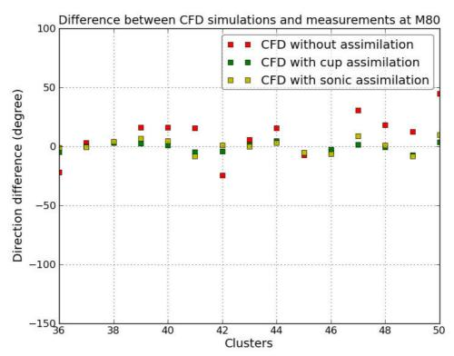
Figure 5.7: Difference between CFD simulations without assimilation and measurements, CFD simulations with cup assimilation and measurement and CFD simulations with sonic assimilation and measurement at M80 (80m) a) wind speed b) direction.
