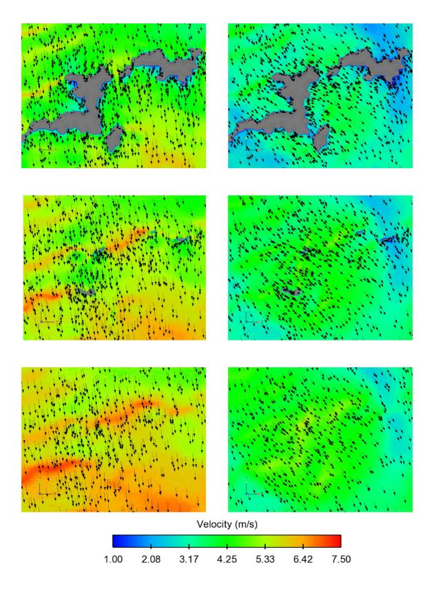
Figure 4.15: Zoom of velocity magnitude and vector cross-section for (a-c) CFD simulation without assimilation and (d-f) CFD simulation with assimilation.
