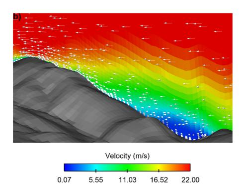
Figure 4.2: Wake formation behind the hill for (a) coarse grid (b) fine grid
