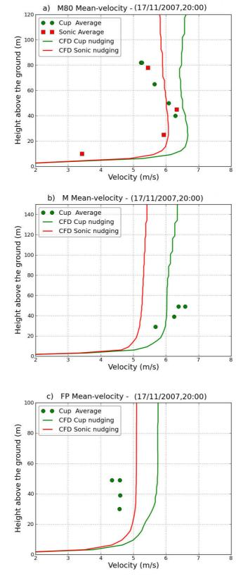
Figure 5.6: Comparison of velocity profile between hourly averaged measurements, CFD simulations with cup and sonic assimilation at M80, M and FP location.
