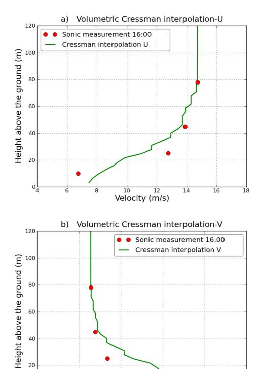
Figure 4.8: Volumetric Cressman interpolation at M80 mast location using sonic anemometer measurement: a) u velocity component and b) v velocity component.
