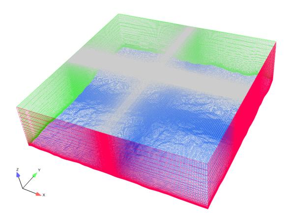
Figure 3.11: Surface grid of the computational domain.
