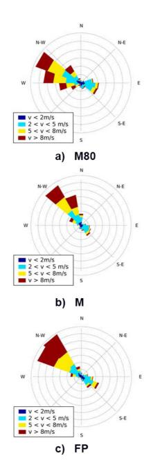
Figure 3.3: Wind rose and magnitude from cup anemometer measurements at a) M80, b) M and c) FP
