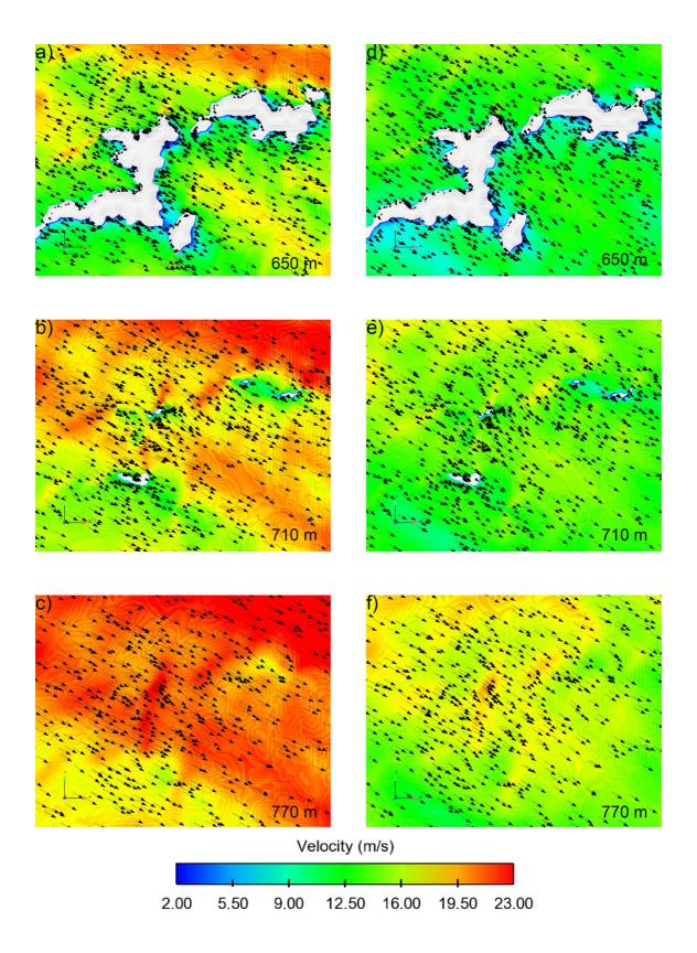
Figure 4.12: Zoom of velocity magnitude and vector cross-section for (a-c) CFD simulation without assimilation and (d-f) CFD simulation with assimilation.
