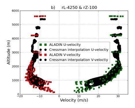
Figure 4.4: Imposed inflow along the north and west boundary using Cressman interpolation for a)  $r_L$ =2000 m and  $r_Z$ =100 m b)  $r_L$ =4250 m and  $r_Z$ =100 m.
