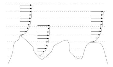
Figure 3.12: Translation coupling method on complex terrain.
