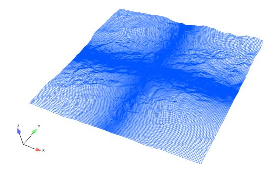
Figure 3.10: Surface mesh of the topography.
