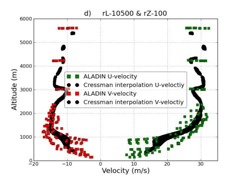
Figure 4.4: Imposed inflow along the north and west boundary using Cressman interpolation for c)  $r_L$ =8500 m and  $r_Z$ =100 m d)  $r_L$ =10500 m and  $r_Z$ =100 m.
