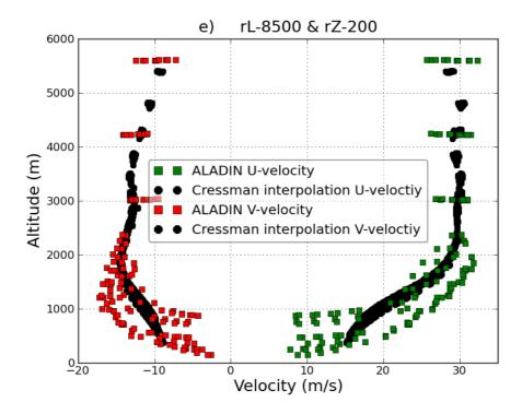
Figure 4.4: Imposed inflow along the north and west boundary using Cressman interpolation for e)  $r_L$ =8500 m and  $r_Z$ =200 m
