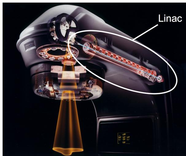
Figure 2.2 – Example of a [linac](#) located in a photon therapy gantry. <sup>1</sup>
