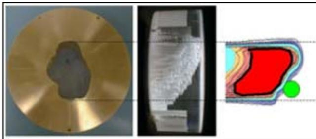
Figure 2.14 – Example of brass aperture and range compensator.<sup>3</sup>
