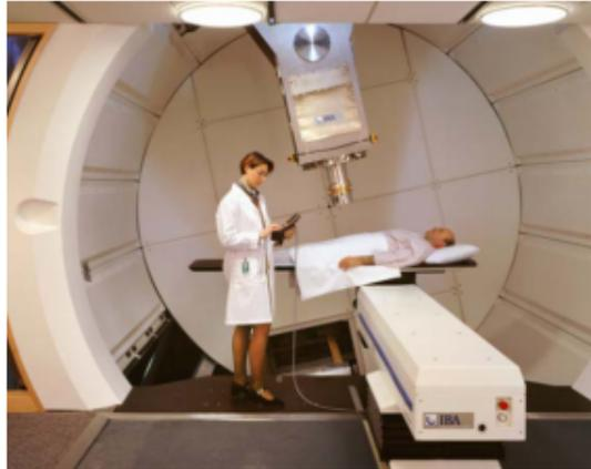
Figure 2.6 – Gantry in a proton therapy treatment room. The nozzle is able to rotate 360 degrees around the movable patient couch. [Paganetti and Bortfeld, 2005]
