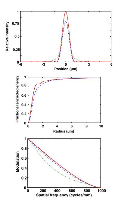
Figure 7.6.: Simulated optical performance of the objective-window system. The PSF (top), fractional encircled energy (middle), and MTF (bottom) are shown both on axis (solid lines) and at  $\pm 245~\mu m$  off axis (dotted and dashed lines, corresponding to in and perpendicular to the plane containing the optical axis and field ray). The ideal performance (dashdotted lines) is included as a reference, but it mostly overlaps with the on axis performance and is only visible in the MTF plot.
