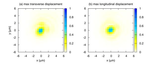
Figure 7.14.: Test 2: the measured PSF at the maximal transverse (off axis) and longitudinal displacement. Apart from the peak intensity reduction, these samples of PSF appear nearly identical to the PSF on axis, indicating a homogeneous performance of the objective over the field of view.
