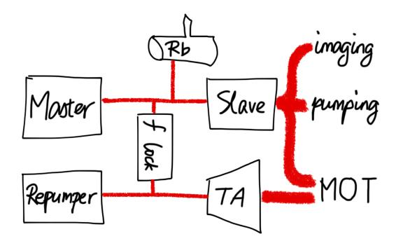
Figure 1.4.: A schematic of the current laser system.
