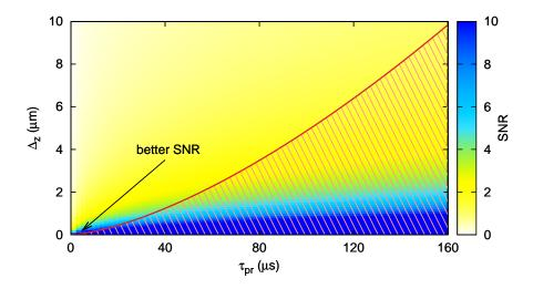
Figure 7.2.: SNR as a function of probe duration  $\tau_{\rm pr}$  and pixel size  $\Delta_z$  at constant saturation parameter s=0.15. The color scale of the SNR is clipped at 10 in order to demonstrate the variation at small SNR.
