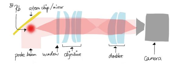
Figure 1.6.: An illustration of the current imaging system.
