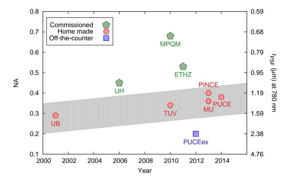
Figure 7.3.: Imaging NA of a few recent experiments with *ex vacuo* optics. The information is obtained mainly from [13] and the references therein, and is therefore by no means exhaustive. The corresponding radius of the central Airy disc evaluated at 780 nm is shown on the right as a reference<sup>a</sup>. The data labels are given here<sup>b</sup>.
