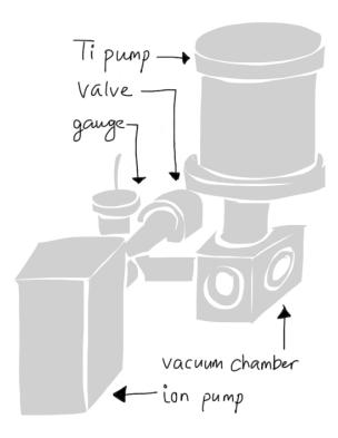
Figure 1.3.: A drawing of the essential components of the vacuum system.
