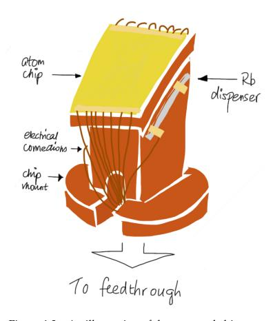
Figure 1.2.: An illustration of the mounted chip.
