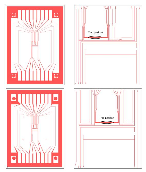
Figure 8.1.: The existing (top) and new (bottom) chip designs. Both the full layout (left) and a zoom (right) showing the atom-trapping wires are shown. The entire chip spans  $2.5 \times 3.5 \text{ cm}^2$ .
