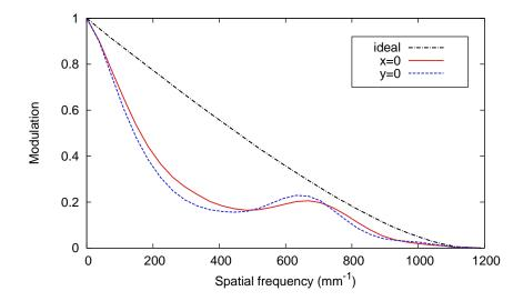
Figure 7.10.: Test 1: the measured modulation transfer function on axis along the two transverse directions *x* and *y* orthogonal to the optical axis. The measurements (solid and dashed lines) are compared with the ideal performance (dash-dotted line). The difference can be explained by a slightly thicker window and the fact that the test is not carried out at the design wavelength.
