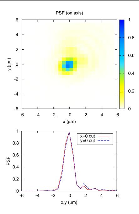
Figure 7.12.: Test 2: the measured PSF on axis and its cuts along x = 0 and y = 0 on axis. The notation is the same as Fig. 7.8. In comparison, the spherical aberration is much reduced at 780 nm. Instead, a slight decentering coma remains, but is uniform throughout the field (see Figs. 7.14).
