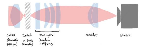
Figure 7.11.: Schematic of the PSF measurement. A microscope slide<sup>a</sup> with submicron pin holes is mounted on a three-axis translation stage, and is illuminated by laser light at 780 nm focused using an asphere<sup>b</sup>. The slide is positioned in the vicinity of the focal point of the window-objective system. A doublet<sup>c</sup> is then used to image the PSF on the camera<sup>d</sup>.
