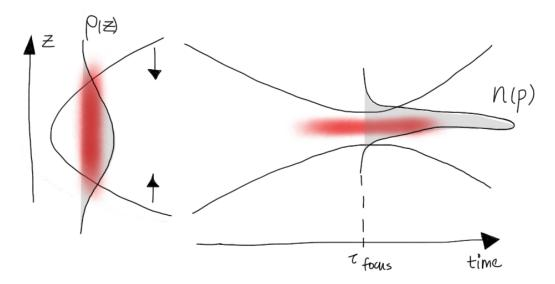
Figure 3.8.: An illustration of the focusing technique. The atoms are focused by a parabolic magnetic field. After a focusing time  $\tau_{TOF}$ , the spatial distribution corresponds to the initial momentum distribution of the atoms.
