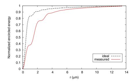
Figure 7.9.: Test 1: the measured normalized encircled energy. The measurement (solid line) on axis is compared with ideal performance (dash-dotted line). The difference can be explained by a slightly thicker window and the fact that the test is not carried out at the design wavelength.
