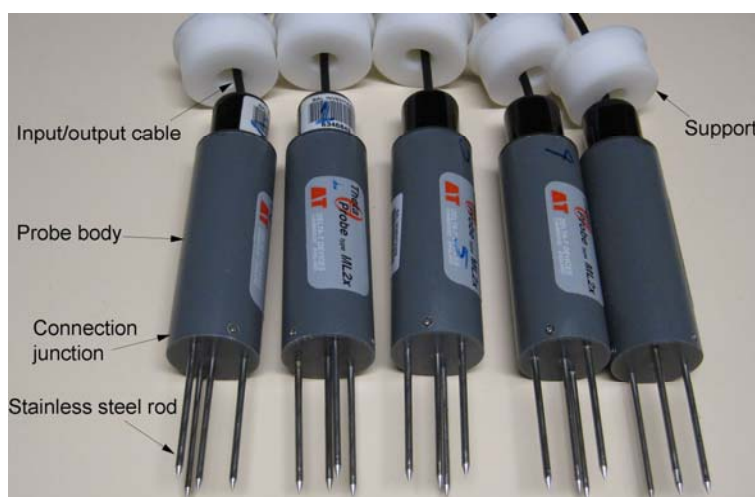
Fig. 2.33. A photograph of ThetaProbe sensors with their supports
