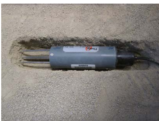
(f) ThetaProbe installation
