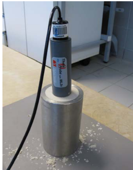
Fig. 2.34. The calibration of ThetaProbe in Fontainebleau sand
