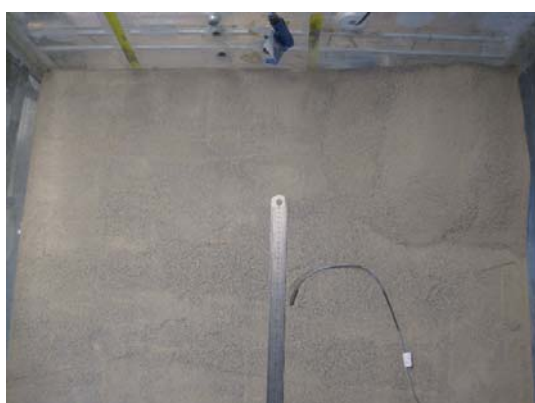
(e) PT1000 installation
