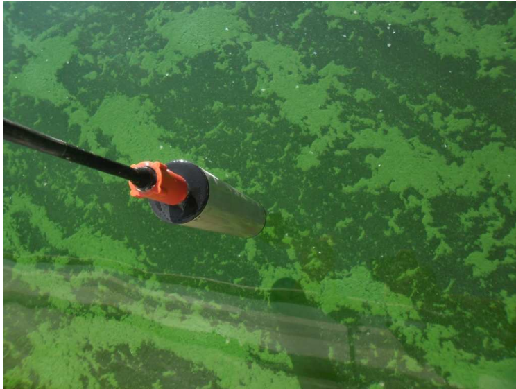
Figure 68 TriOS microFlu-blue at Karaoun Reservoir
