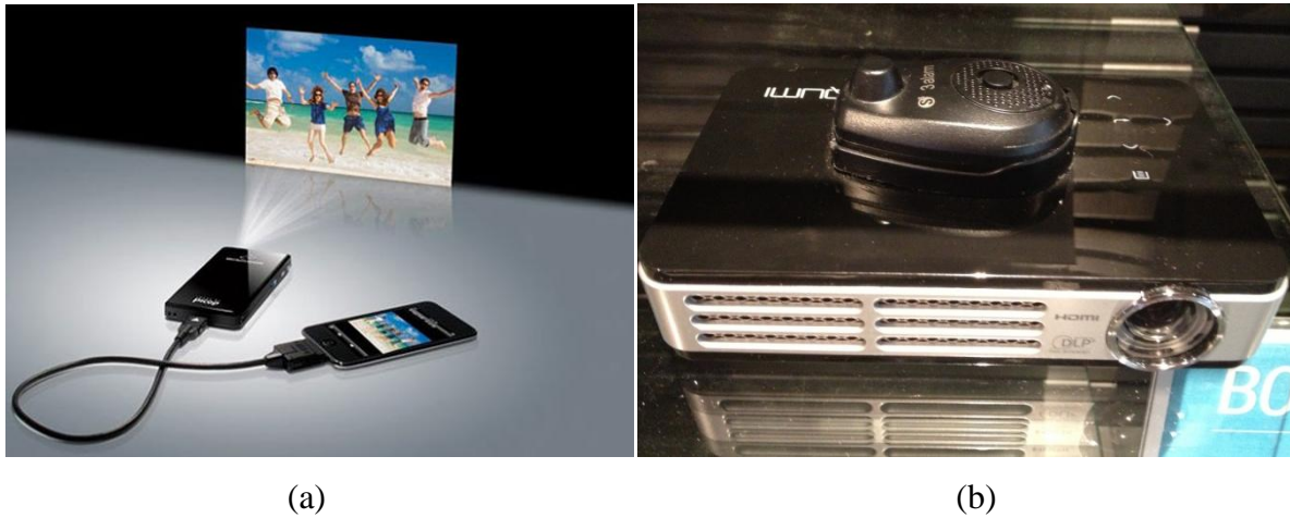
Fig. 17 Micro video projector: (a) for Smartphone; (b) for standard use.
