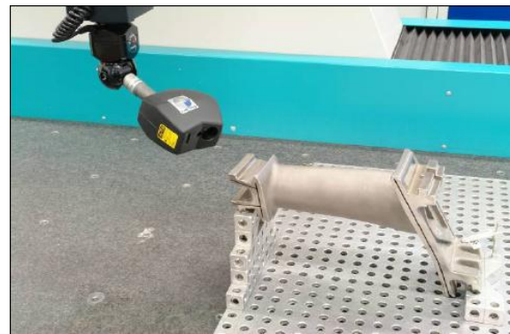
Fig. 2 Turbine blade measurement by laser triangulation scanning (Nikon metrology labs).
