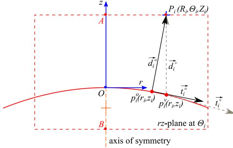
Fig. 74 Orthogonal/vertical distance vector from a data point  $P_i$  to its footpoint  $p_i^o/p_i^v$  on an asphere is contained in the  $rz$ -plane at an angle  $\theta_i$  passing through the axis of symmetry (red points O, A, B,  $P_i$ ,  $p_i^o$  and  $p_i^v$  are coplanar): planar view in the  $rz$ -plane.
