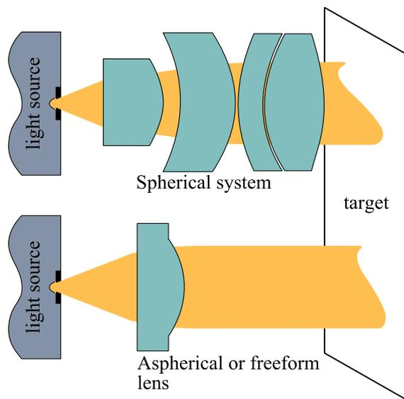
Fig. 16 Aspherical lens based systems replacing spherical systems.
