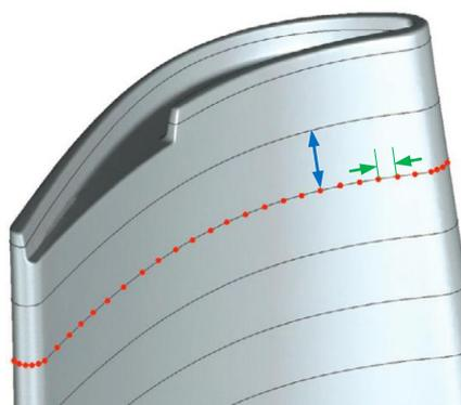
Fig. 143 Scanning of the turbine blade in lines of scan. Lateral point spacing (blue) is much larger than longitudinal spacing (green).
