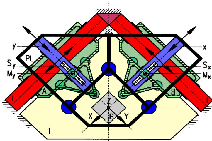
Fig. 33 Schematic of the F25 XY platform (Top View). PL: moving platform (thick black);  $x$  and  $y$ :  $x$ - and  $y$ - linear drives;  $S_x$  and  $S_y$ : Ultra-precise glass ceramic length measuring systems with nanometric scales [45].
