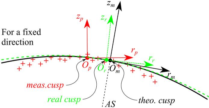
Fig. 60 Illustration of the problem with the alignment of the measurement coordinate system. Indices  $m$ ,  $p$  and  $r$  stand for model, measured point-set and real surface, respectively; AS: theoretical axis of symmetry.
