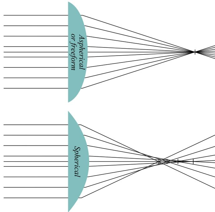
Fig. 15 Aspherical and freeform optics reduce spherical aberrations [57].
