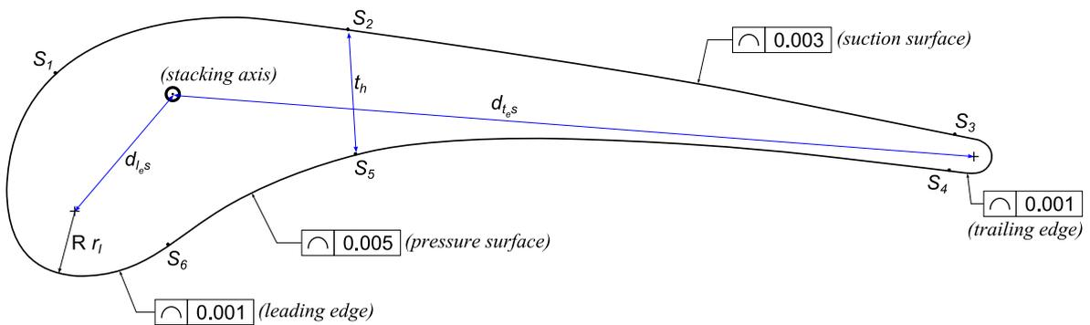
Fig. 22 Geometrical tolerancing of a turbine blade profile according to ISO 1101 ( $d_{l_{eS}}$ : leading edge to stacking axis distance;  $d_{t_{eS}}$ : trailing edge to stacking axis distance;  $S_i$ : stacking points;  $r_1$ : leading edge radius of curvature;  $t_h$ : central thickness).
