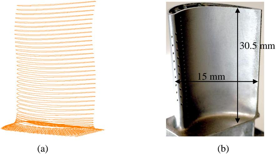
Fig. 63 The turbine blade provided by Geomnia: (a) the measured dataset; (b) the real part.
