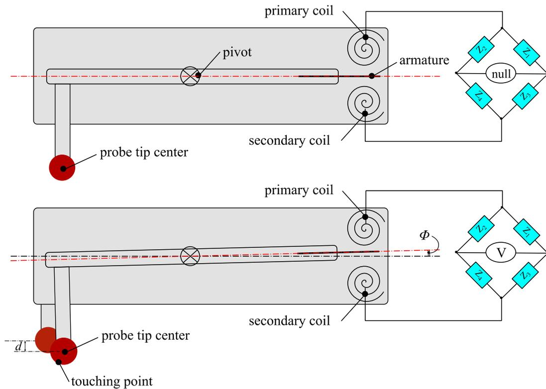
Fig. 51 The stylus probe principle.
