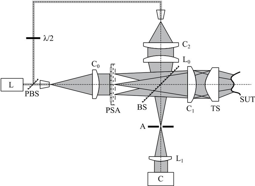
Fig. 46 The Tilted-Wave Interferometer setup. (L: coherent laser source, PBS: polarizing beam splitter, BS: beam splitter, C<sub>0,1,2</sub>: collimators, PSA: micro-lens array followed by a pinhole array, L<sub>0,1</sub>: imaging optical lens, TS: transmission sphere, SUT: Surface Under Test) [96].
