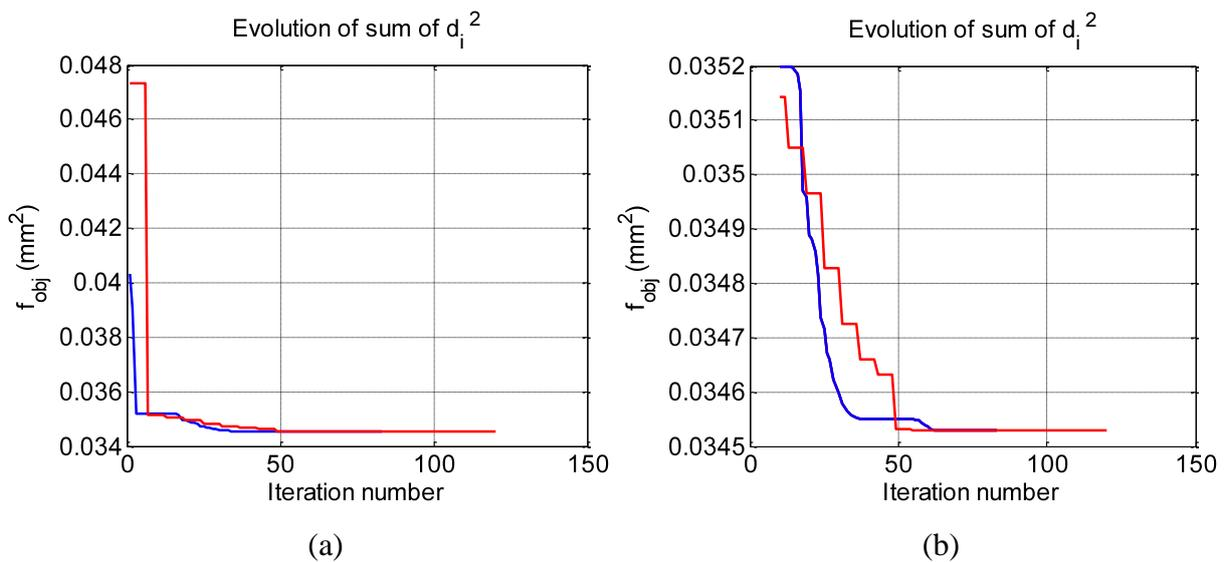
Fig. 91 Evolution of the objective function value through the iterations for the case of  $T\text{Scan}_1$  (legend: L-BFGS: blue, LM: red,  $f_{\text{obj}} = \phi$ ). (a) All iterations; (b) Starting from iteration 10.
