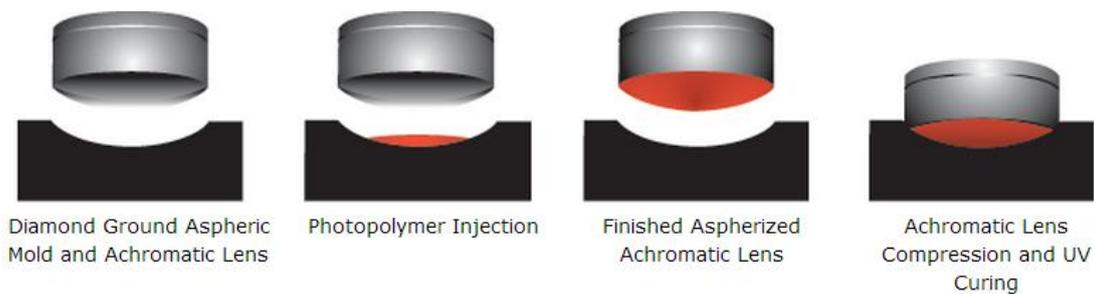
Fig. 28 Aspheres molding [84].
