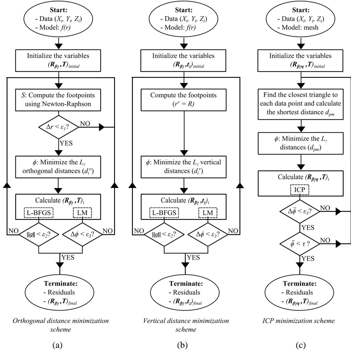
Fig. 73 Sequential algorithm for the fitting problem.  $L_2$ : Least-Squares norm;  $\mathbf{R}_{\beta\gamma}$  or  $\mathbf{R}_{\beta\gamma\eta}$ : combined rotation matrix and  $\mathbf{T}$ : translation vector;  $\Delta\phi$ : change in the objective function value;  $\|g\|$ : norm of the gradient of  $\phi$ ;  $\varepsilon_1, \varepsilon_2, \varepsilon_3$ : the algorithms stop criteria;  $\tau$ : ICP convergence tolerance.
