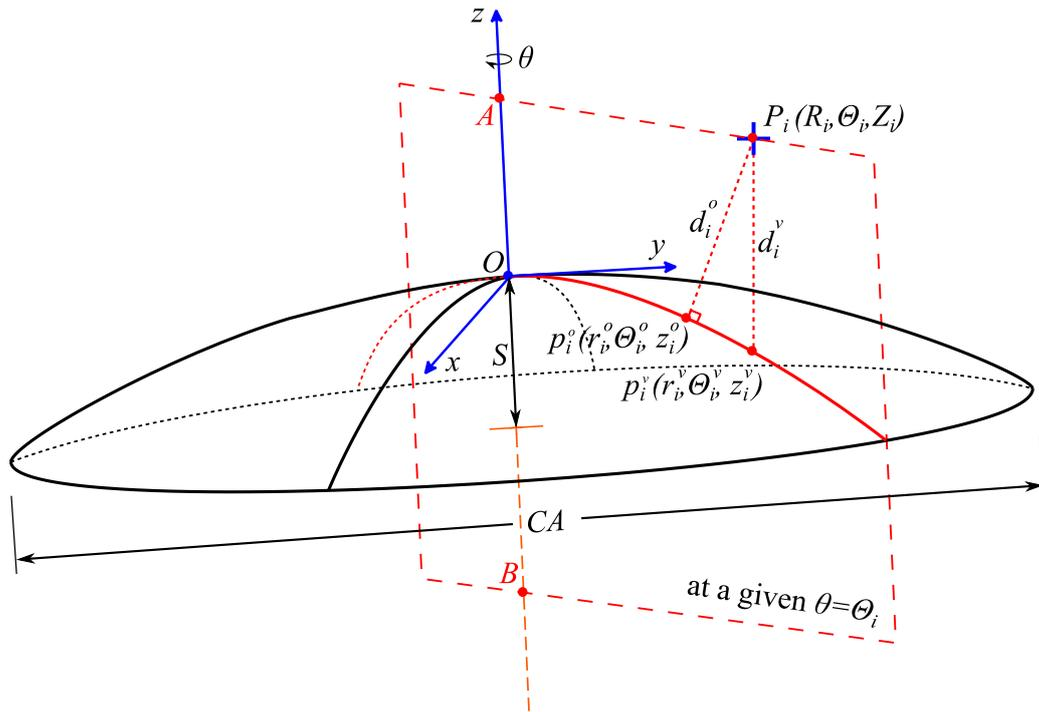
Fig. 68 Orthogonal/vertical distance vector from a data point  $P_i$  to its footpoint  $p_i^o/p_i^v$  on an asphere is contained in the  $rz$ -plane (red) at an angle  $\theta_i$  passing through the axis of symmetry (points O, A, B,  $p_i^o$  and  $p_i^v$  are coplanar).
