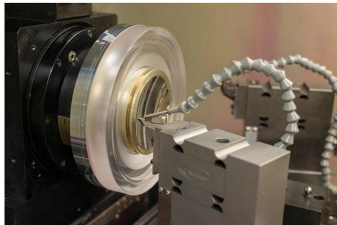
Fig. 23 Single Point Diamond Turning from Empire Precision.
