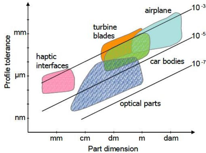
Fig. 18 Tolerance versus part dimension of freeform surfaces [8].
