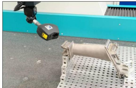
Fig. 2 Turbine blade measurement by laser triangulation scanning (Nikon metrology labs).
