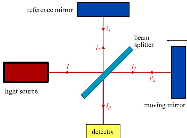
Fig. 58 The Michelson interferometer.
