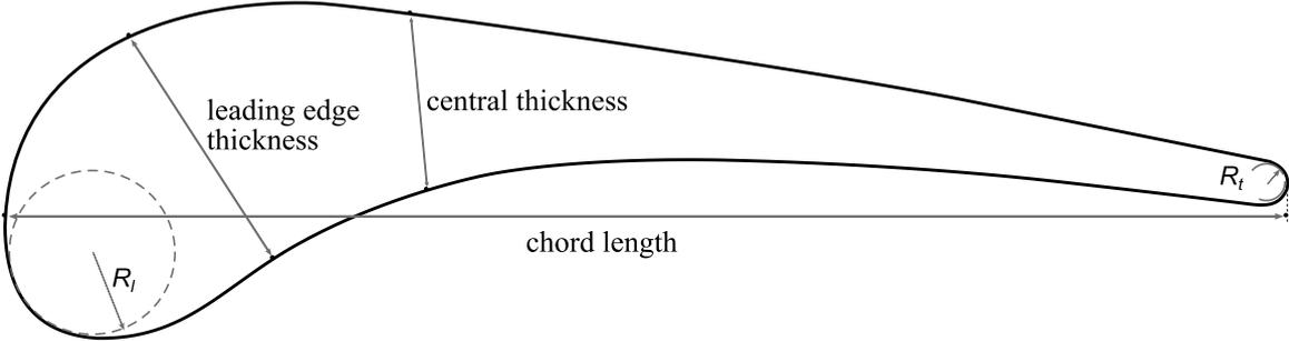
Fig. 6 Some geometrical dimensions defined on a turbine blade profile ( $R_l$ : leading edge radius of curvature;  $R_t$ : trailing edge radius of curvature).
