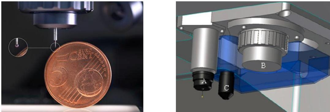
Fig. 34 (a) Tactile probe of the F25 machine; (b) conceptual design and layout of the tactile (A) and confocal (C) probes mounted on F25 [89].
