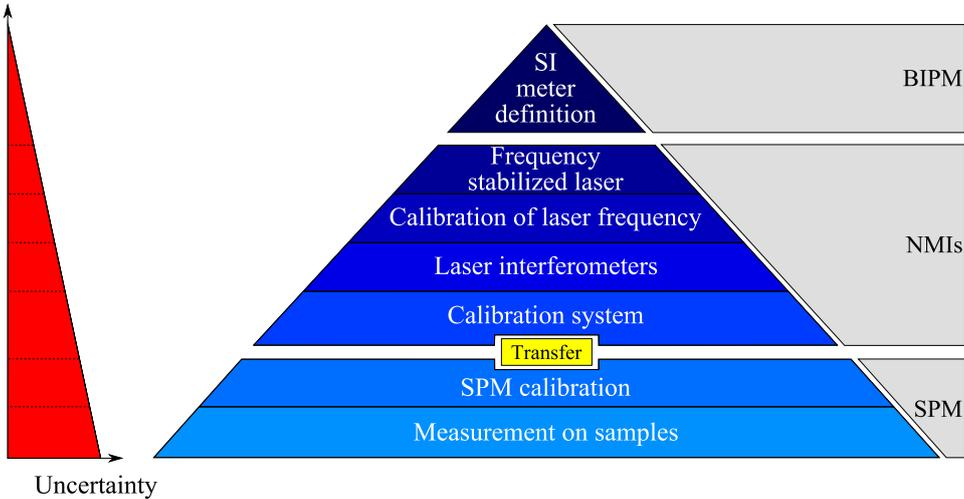
Fig. 3 Metrology traceability pyramid (SPM: Scanning Probe Measurement).
