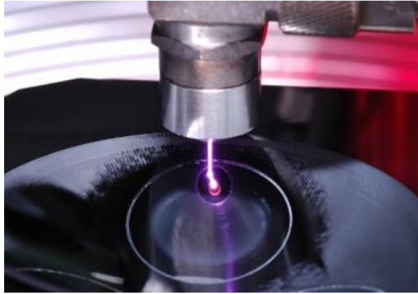
Fig. 25 Ion and plasma beam machining from TNO.
