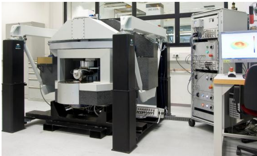
Fig. 39 NANOMEFOS non-contact measurement machine for freeform optics [2].
