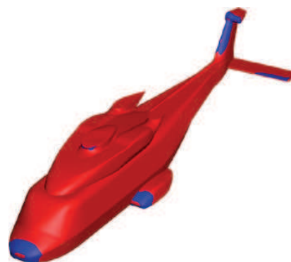
Fig. 10 Laminar region ( blue ) computed using the Langtry–Menter two-transport equations for the transition prediction
