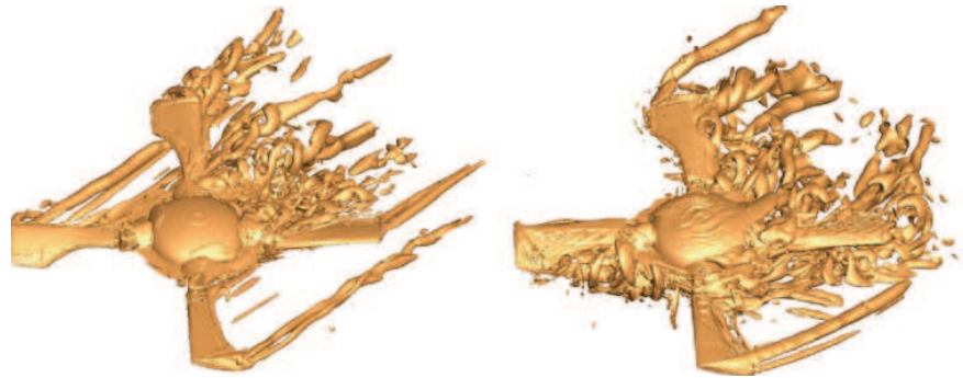
Fig. 12 Isosurface of Q-criterion for steady (left) and unsteady (right) computations
