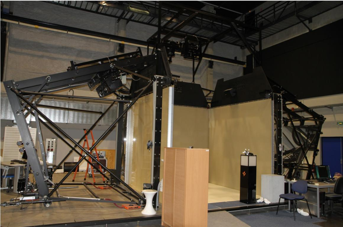
Figure 3.45: Our CAVE system (multi-screen display system) ( $3 \times 3$  meters across).
