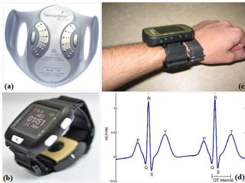
**Figure 4.4:** (a) Example of metallic sensors<sup>2</sup>, (b) wireless heart rate sensor<sup>Garmin</sup>, (c) blood pressure sensor<sup>140</sup>, (d) typical ECG signal for a healthy person.
