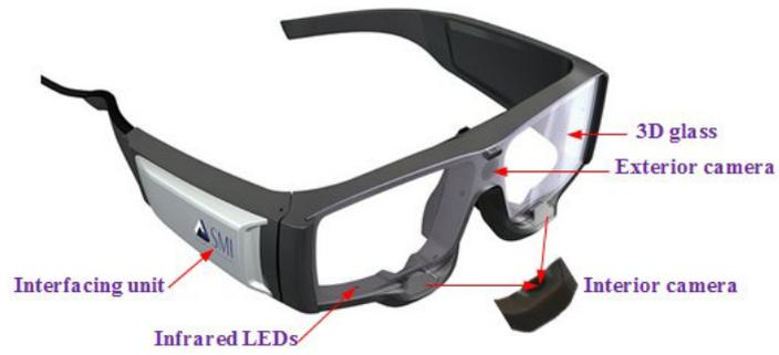
Figure 6.20: SMI eye tracking sensor.
