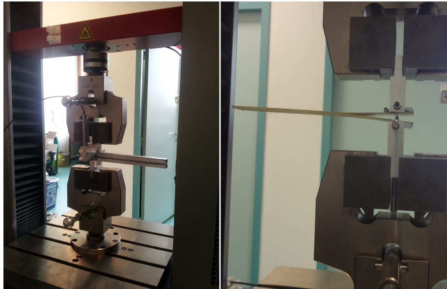
Figure 4.28. Experimental setup for Double Cantilever Beam test (a) Aluminium substrate and (b) Kevlar composite with end blocks
