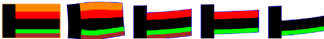
Figure 1.32: The Multi-step procedure with predetermined material removal [99]
