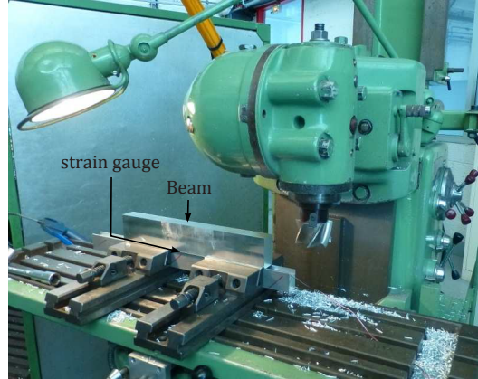
Figure 3.2: The experimental set-up used to perform the layer removal method
