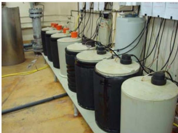
Figure 2.2: Circulating natural sea water tanks.
