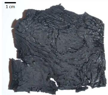
Figure 6.2: Crack formation on polychloroprene surface after 6 months at 80°C in sea water.
