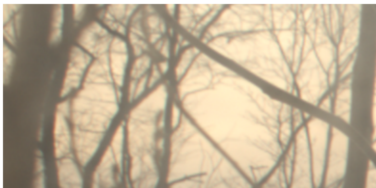
Figure 4.2: Example of LCA presence in digital image crop taken by camera Sony DSLR-A200 with focal length f = 24mm . The color channel misalignments are noticeable due to LCA and are mostly highlighted in the regions of edges.
