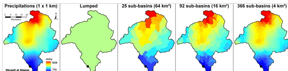
**Figure 44 :** Distributed precipitation forcing (10-year average) for the catchment discretizations of the Héroult catchment at Gignac (1430 km<sup>2</sup>) shown in Figure 26.
