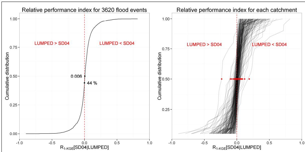
**Figure 51 : Distribution of relative performance index values in validation mode between the lumped model and the SD04 semi-distributed model. The distribution is drawn for the whole set of 3620 flood events (left) and for the 20 events of each catchment (right). The red points show the median values of the relative performance index for each catchment.**
