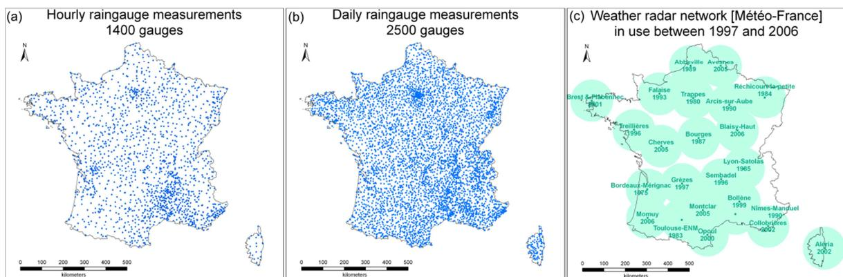
**Figure 40 : Structures of the operational measurement network for precipitation estimates between 1997 and 2006. (a) automatic hourly rain gauge network ; (b) daily manual rain gauge network; (c) Theoretical coverage of the weather radar (location name and year of installation are indicated).**
