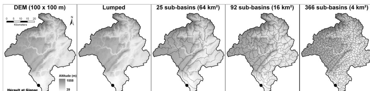
**Figure 43 :** Example of lumped and semi-distributed catchment discretizations (with unit sizes of 64, 16 and 4 km<sup>2</sup>) for the Héroult catchment at Gignac (1430 km<sup>2</sup>).
