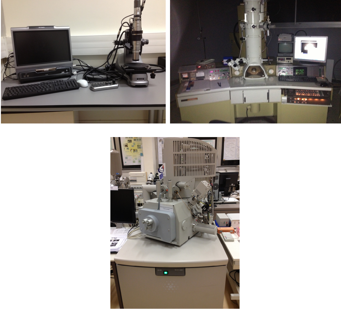
Figure A.6 - (a) Microscope optique VHX-1000 (KEYENCE) ; (b) MET JEOL 2000 ; (c) MEB Quanta 600 FEG (FEI).
