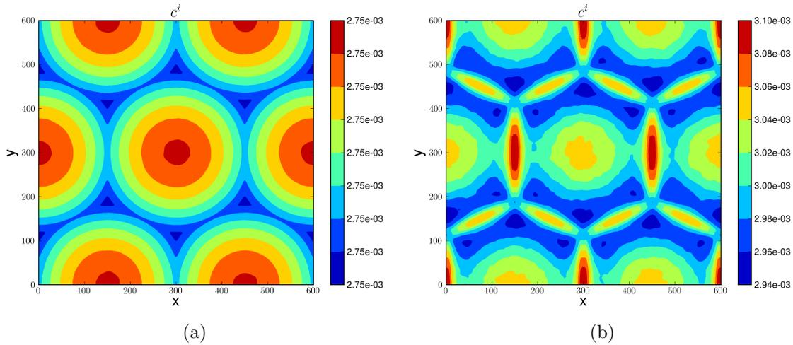
Figure 4.9: Predicted SIA distribution of an irradiated Fe polycrystal after 1 dpa, using (a) constant parameters ( $D_i, D_v$  and  $K_{iv}$ ) and (b) effective parameters
