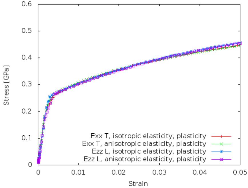
Figure 5.11: Stress strain curve for a Cu-Nb bilayer, simulated in tension along two orthogonal directions contained in the interface plane.
