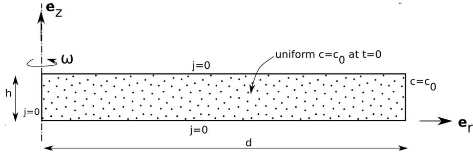
Figure 2.1: Definition of the rotating disc set-up: geometry, boundary conditions and mechanical loading.
