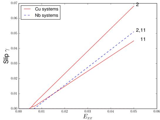
(c) Slip on every system in a Cu-Nb multilayer, for Case D
