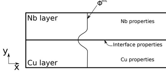
Figure 5.4: Finite element modeling of a Cu-Nb system. Each layer is represented by a set of material points. A diffuse field,  $\phi^{int}$ , is used to interpolate the single crystal and the interface properties.
