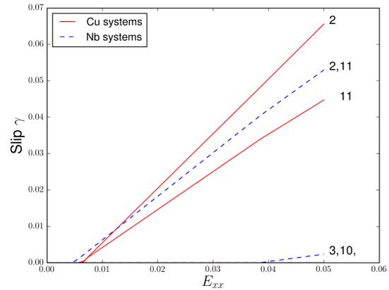
(d) Slip on every system in a Cu-Nb multilayer, for Case D (ARB), using elastic anisotropy.
