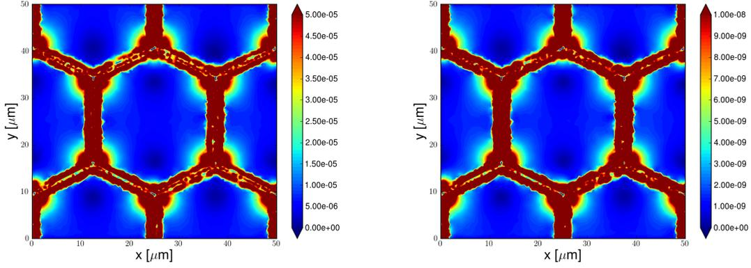
(a) Equivalent diffusional inelastic strain ( $t = 5 \times 10^3$ s).
