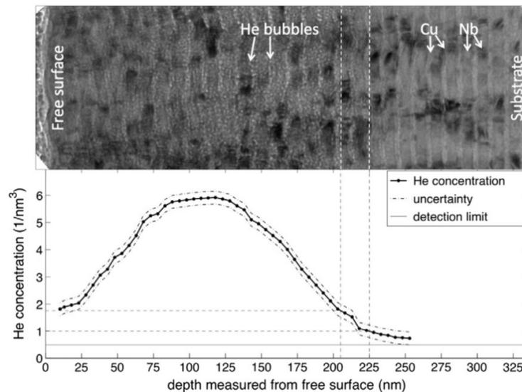
Figure 1.2: A comparison between the TEM micrograph of a  $\text{He}^3$ -implanted Cu–Nb multilayer (top) and the corresponding He concentration profile measured by Nuclear Reaction Analysis (bottom) reveals a critical depth at which no He bubbles are observed (indicated by dashed lines), even though the He concentration is not zero. [38]
