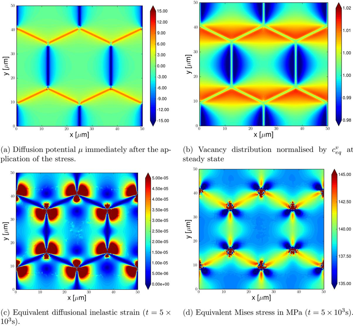
Figure 3.4: (a) Diffusion potential, (b) vacancy distribution, (c) inelastic strain and (d) equivalent Mises stress in the case of Dirichlet boundary conditions, with an applied stress of 80 MPa and a  $25\mu\text{m}$  grain size, and for isotropic elasticity. The mechanical effect on the diffusion potential is clearly visible in (a): the location of each grain boundary is revealed by a different diffusion potential value, depending on the GB orientation.
