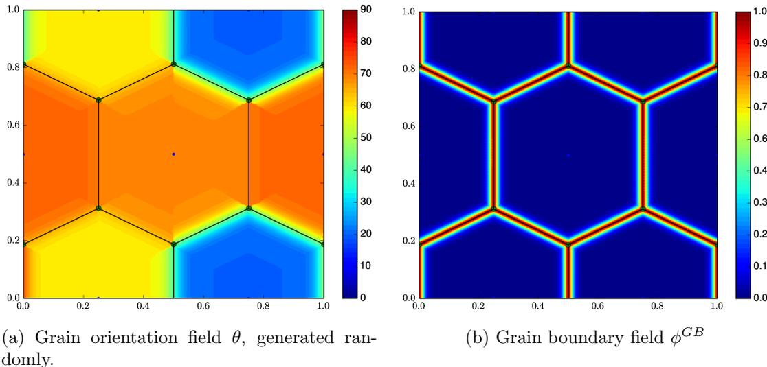
Figure 3.2: Periodic 2D polycrystal aggregate used in the simulations. The window size is varied from 20 to 200  $\mu\text{m}$ . The edges of the Voronoi cells are superimposed to the fields.
