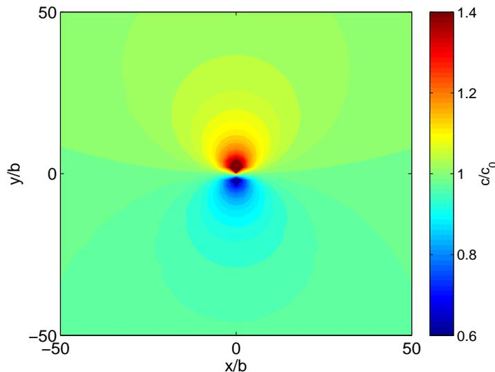
Figure 2.5: Contour plot of the numerically obtained equilibrium vacancy concentration distribution normalised by  $c_0$ . The vacancies tend to relieve the hydrostatic pressure around the dislocation core by migrating from the tensile regions to the compression ones.
