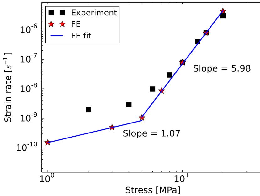
Figure 3.10: Strain rate dependence on stress. Data taken from [127].
