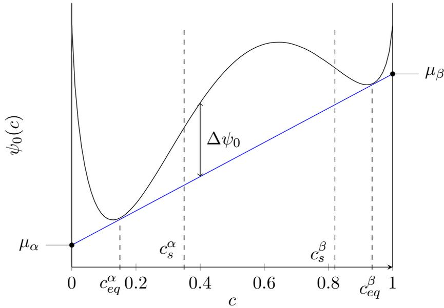
Figure 4.2: Example of a non-convex homogeneous chemical free energy,  $\psi_0$ . The two minima are denoted  $c_{eq}^\alpha$  and  $c_{eq}^\beta$ . The two convex wells are separated by a non convex region, delimited by the spinodal points  $c_s^\alpha$  and  $c_s^\beta$ .
