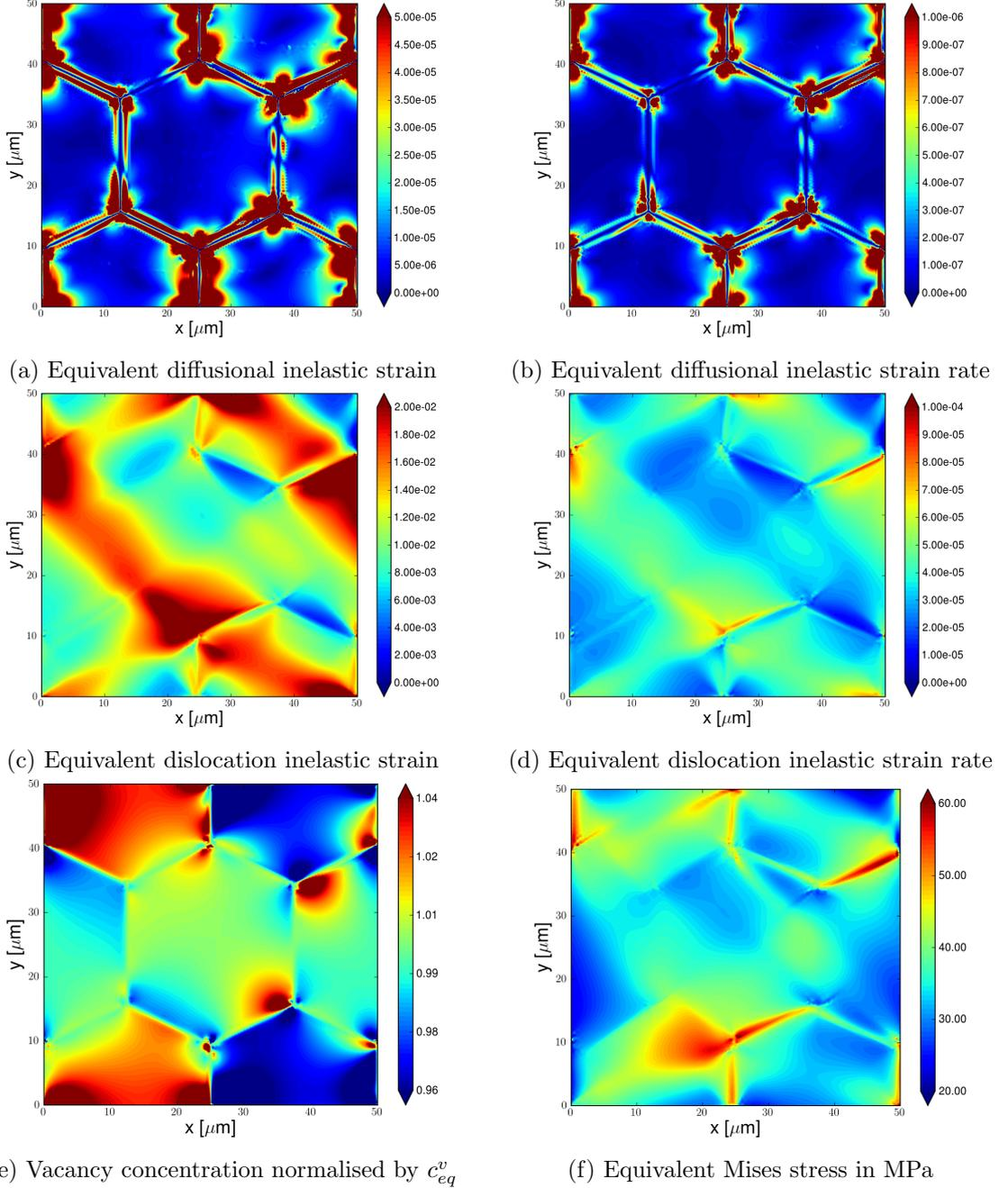
Figure 3.9: Inelastic (a) diffusional strain, (b) diffusional strain-rate, (c) dislocation strain, and (d) dislocation strain-rate, and (e) vacancy concentration and (f) equivalent Mises stress (applied stress of 20 MPa,  $25\mu\text{m}$  grain size and at  $t = 3.10^3\text{s}$ )
