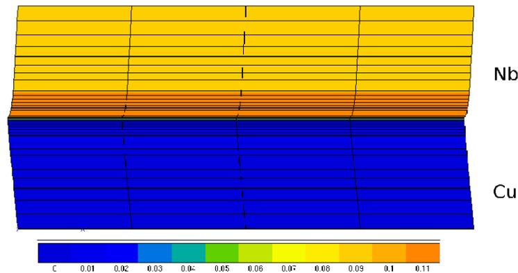
Figure 5.15: Accumulated plastic strain for an imposed mean shear strain of  $E_{xy}=0.05$ , for the case of a shearable interface. The plastic activity is more intense in the niobium layer, close to the interface.
