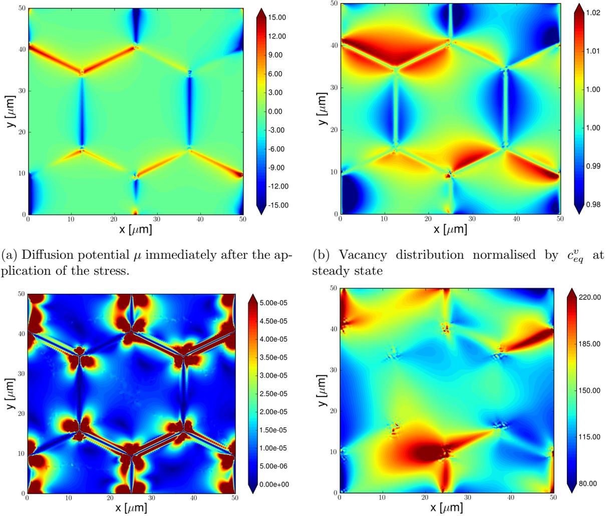
(a) Diffusion potential  $\mu$  immediately after the application of the stress.
