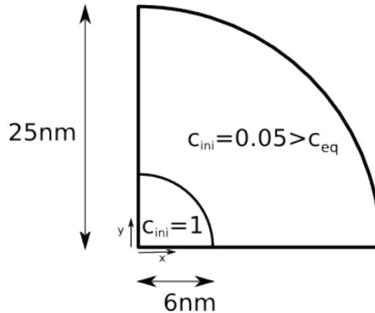
Figure 4.6: Single void growth simulation set-up. An initial void of radius 6 nm is placed in a vacancy supersaturated matrix, and symmetry conditions are applied at  $x=0$  and  $y=0$ . A no-flux condition is imposed on the outer arc.
