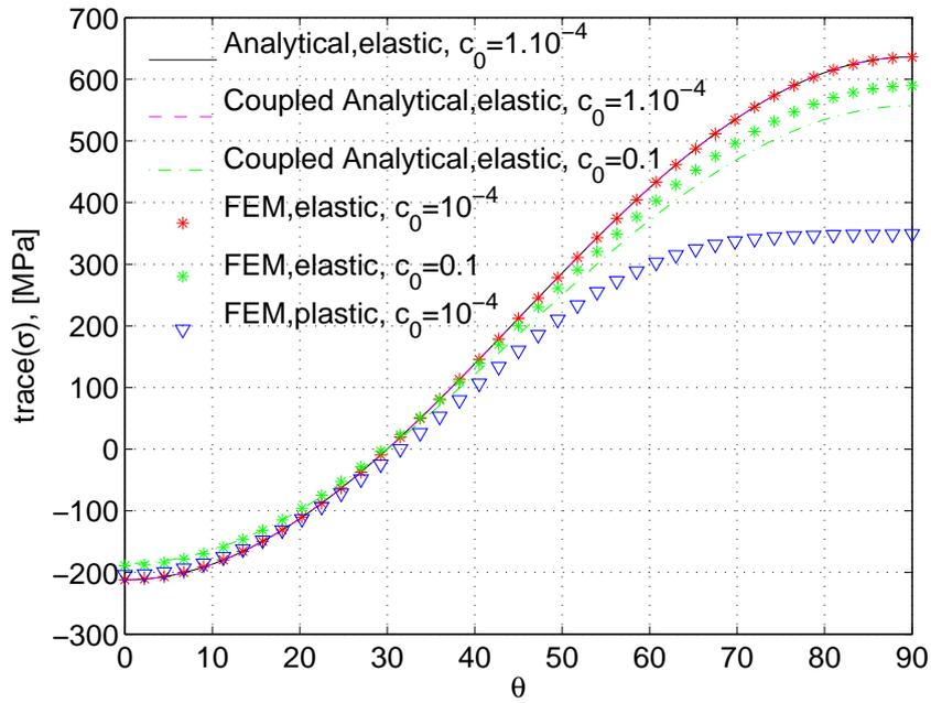
Figure 2.7: Variation of the trace of the stress tensor around the hole for two different values of initial vacancy concentration, without and with the effect of the open system (ie, coupled) elastic constants. The effect of the concentration on the stress is noticeable for high concentrations.
