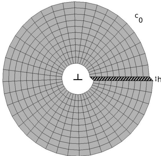
Figure 2.3: Model of the edge dislocation problem (deformed configuration, zoomed on the core): an eigenstrain  $\varepsilon_{12}^* = -\frac{b}{h}$  is imposed in the stripped zone, and a cutout of radius  $2b$  is made to exclude the core, with a vanishing flux boundary condition. A concentration  $c_0$  is imposed on the far-field boundaries.
