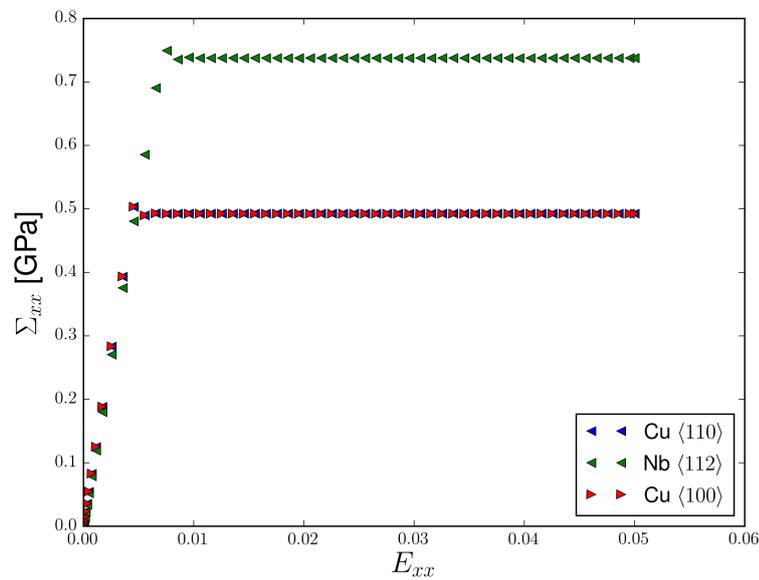
Figure 5.6: Simulated tensile stress-strain curves for elastically isotropic single crystals. The curves for single crystal Cu are identical for Case B  $\langle 100 \rangle$  and C  $\langle 110 \rangle$  orientations.
