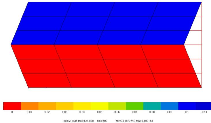
Figure 5.13: Accumulated plastic strain, for an imposed mean shear strain of  $E_{xy}=0.05$ , in the deformed shape.
