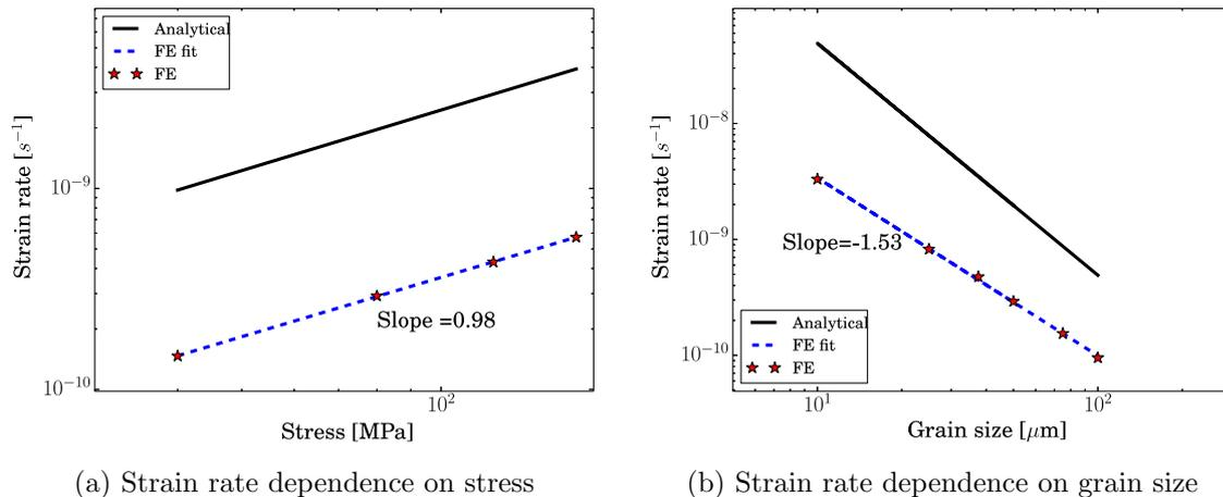
Figure 3.8: Comparison between the macroscopic Herring-Nabarro creep law and the finite element simulation results using a source term in the grain boundary of width  $4\mu\text{m}$ . According to the analytical solution eq. (3.46), the slopes in figures (a) and (b) should have value of 1 and  $-2$ , respectively.
