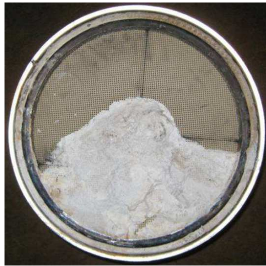
(b) SCR catalyst with solid deposit.
