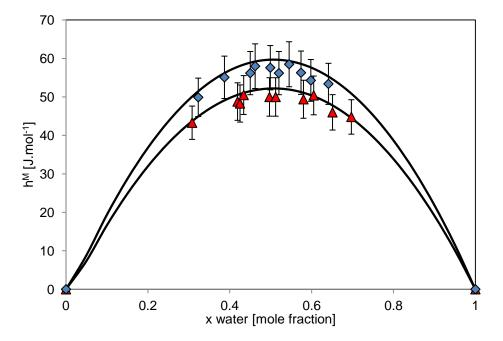
Figure 5.29: Enthalpies of mixing at atmospheric pressure of the binary system water – propane at 383.2 K ( $\blacklozenge$ ) and 393.2 K ( $\blacktriangle$ ) [5.39]. (-) GC-PR-CPA model. Error bar: ± 10%.
