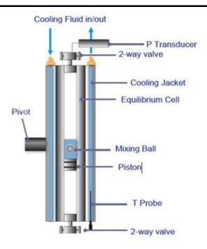
Figure 2.2: Schematic of apparatus used for bubble point measurements.
