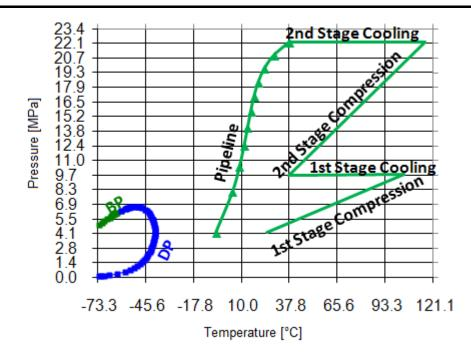
Figure 1.9: Natural gas phase envelope and compression conditions [1.18]
