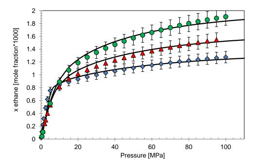
*Figure 5.1: Ethane solubility in water at 313.15 K* ( $\blacklozenge$ ), *373.15 K* ( $\blacklozenge$ ) *and 393.15 K* ( $\bullet$ ) **[5.6]**. (-) *GC-PR-CPA model. Error bar:*  $\pm 7\%$
