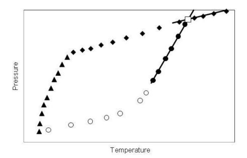
Figure 2.7: Pressure – temperature diagram for estimating hydrate dissociation point.  $\blacklozenge$  thermal expansion,  $\blacktriangle$  pressure drop (hydrate formation),  $\circ$  heating,  $\bullet$  step by step heating,  $\Box$  hydrate dissociation point
