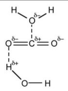
*Figure 3.6: Water solvation of carbon dioxide* [3.26].
