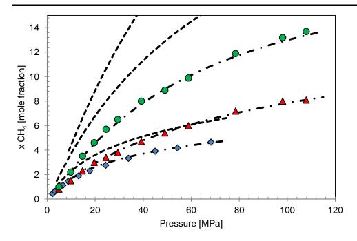
Figure 4.1:  $CH_4$  solubility in water at 310.93 K ( $\diamond$ ) [4.4], 423.15 K ( $\blacktriangle$ ) and 473.15 K ( $\bullet$ ) [4.5]. - SRK–CPA EoS with  $k_{ij}=0$ . - SRK–CPA EoS with adjusted  $k_{ij}$ .
