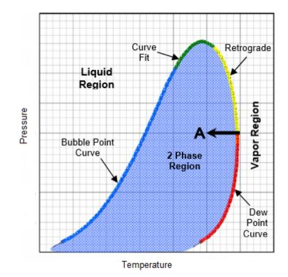
*Figure 1.7: Example of natural gas phase diagram* [1.14]
