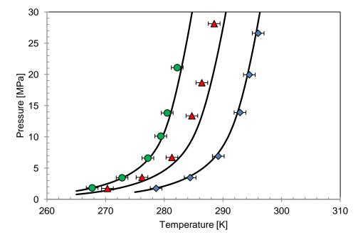
Figure 5.27: Hydrate dissociation points of MIX 5 with deionised water ( $\blacklozenge$ ), 25%<sub>wt</sub> ethanol ( $\blacktriangle$ ) and 25%<sub>wt</sub> methanol ( $\bullet$ ). (-) GC-PR-CPA model. Error bar: ±0.5 K.
