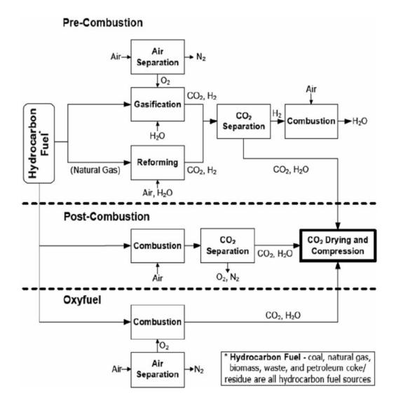
*Figure 1.12: Schematic of processes for carbon dioxide capture* **[1.9**].
