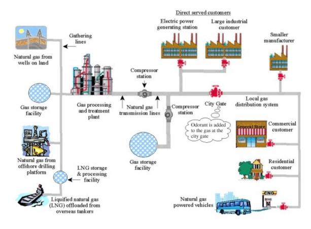
Figure 1.8: Natural gas pipeline network [1.15]
