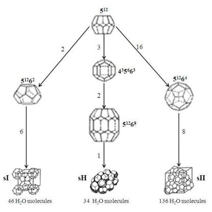
*Figure 1.16: Hydrates structures* [1.40]
