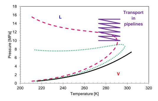
Figure 1.14: Phase diagram for different  $CO_2 - N_2$  mixtures ( \_\_\_\_\_) 99.99%<sub>mol</sub>  $CO_2+0.01\%_{mol}N_2$ . ( \_\_\_\_\_\_) 90%<sub>mol</sub>  $CO_2+10\%_{mol}N_2$ . ( \_\_\_\_\_\_) 80%<sub>mol</sub>  $CO_2+20\%_{mol}N_2$ .
