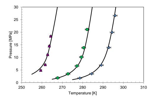
Figure 5.28: Hydrate dissociation points of MIX 5 with deionised water ( $\blacklozenge$ ), 25%<sub>wt</sub> methanol ( $\blacklozenge$ ) and 50%<sub>wt</sub> methanol ( $\blacktriangle$ ). (-) GC-PR-CPA model. Error bar: ±0.5 K.
