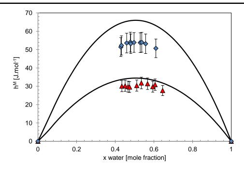
Figure 5.31: Enthalpies of mixing at atmospheric pressure of the binary system water – nitrogen at 373.15 K ( $\blacklozenge$ ) and 423.15 K ( $\blacklozenge$ ) [5.41]. (-) GC-PR-CPA model. Error bar: ± 10%.
