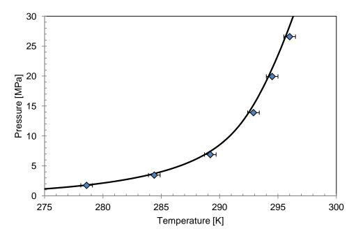
*Figure 5.26: Hydrate dissociation points of MIX 5 with deionised water. (-) GC-PR-CPA model. Error bar:* ±0.5 *K.*
