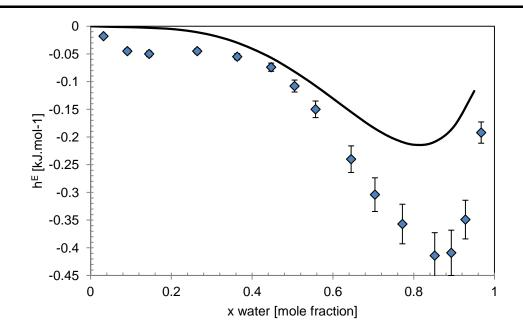
*Figure 5.32: Excess enthalpies at atmospheric pressure of the water – ethanol binary system at 323.15 K* **[5.43]**. (-) *GC-PR-CPA model. Error bar:* ± 10%.
