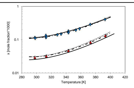
Figure 5.8: Toluene (♦) and Ethylbenzene (▲) solubilities in water at 0.5 MPa [5.17].
