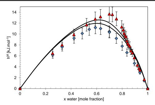
Figure 5.30: Enthalpies of mixing at 16.4 MPa of the binary system water – benzene at 581 K ( $\diamond$ ) and 592 K ( $\blacktriangle$ ) [5.40]. (-) GC-PR-CPA model. Error bar: ± 10%.
