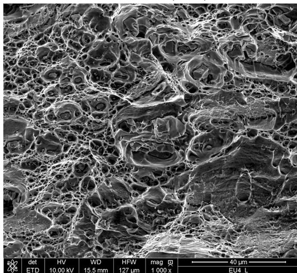
*EU<sub>4</sub>* sens L (1000x)
