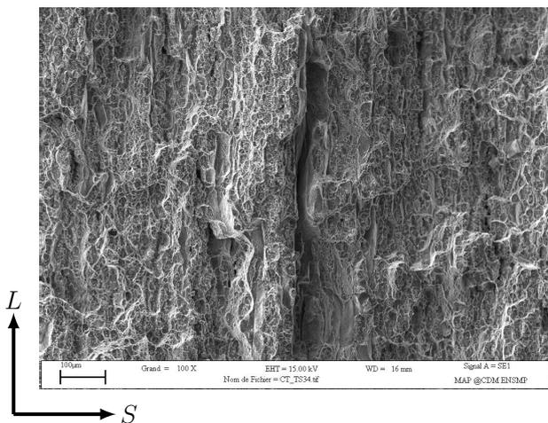
Eprouvette CT10 sens  $T - S$  (100x)
