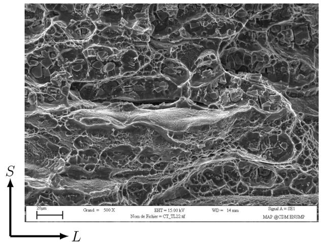
Eprouvette CT10 sens  $T - L$  (500x)
