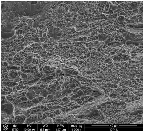
*DP sens L (1000x)*
