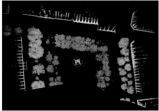
(b) St. Sulpice square: elevation image from the upper slice: points higher than H_{\text{slice}} .
