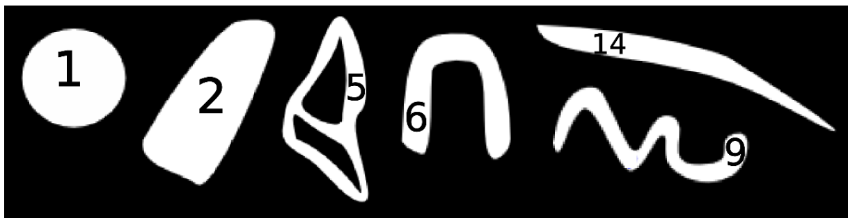
Figure 7.4: Geodesic elongation for different binary objects. The elongation values have been approximated to get integer values. The longer and narrower the object, the higher the elongation. The lowest bound is reached with the disk, where E(\text{disk}) = 1 . In this image, the number on each object corresponds to its approximated elongation. An efficient implementation can be found in Morard et al. (2013) .
