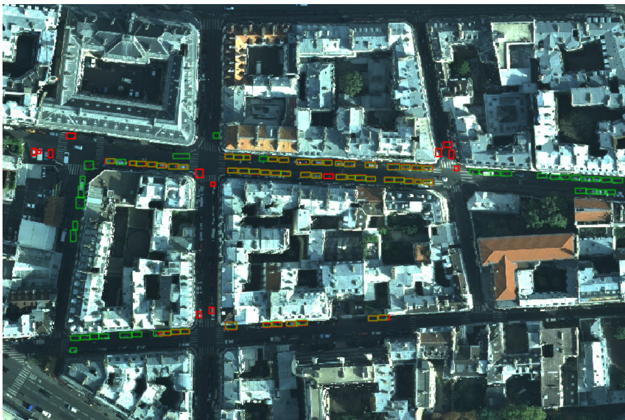
(b) Classification results exported to a GIS. Cars detected in the first passing (red), in the second (green), in both (orange).
