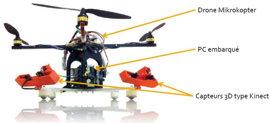
FIGURE 3.1 – Structure du quadrotor
