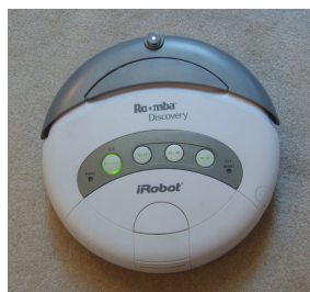
FIGURE 1.2 – Le robot ménager Roomba de IRobot
