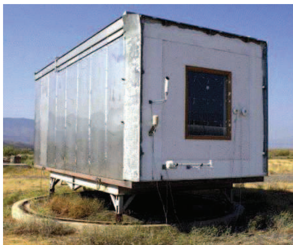
Figure 12 : Cellule test PASSYS [31].
