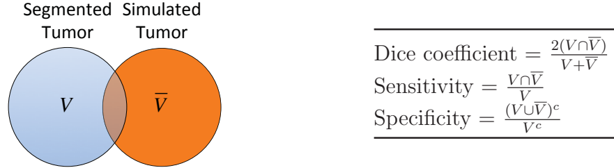
Figure 4.4: Dice coefficient, Sensitivity, and Specificity definitions between segmented and simulated tumor volumes, represented by V and \bar{V} respectively. The Dice coefficient ranges from zero to one, where one means that the simulated and segmented tumors match volumetrically.
