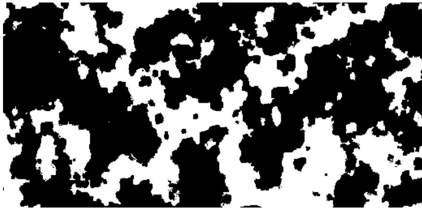
FIGURE 4.12: Slice view of the observed structure obtained from the segmentation of FIB-SEM images of the nanoporous additive.
