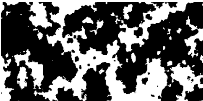
FIGURE 5.7: Segmented FIB-SEM image of the nanoporous additive.
