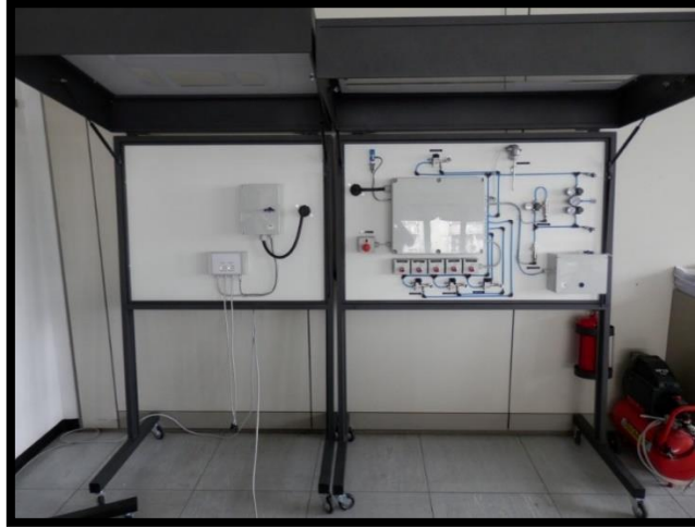
Fig. 3-3. Synoptic panel, a replica of the on-board unit installed in the trucks
