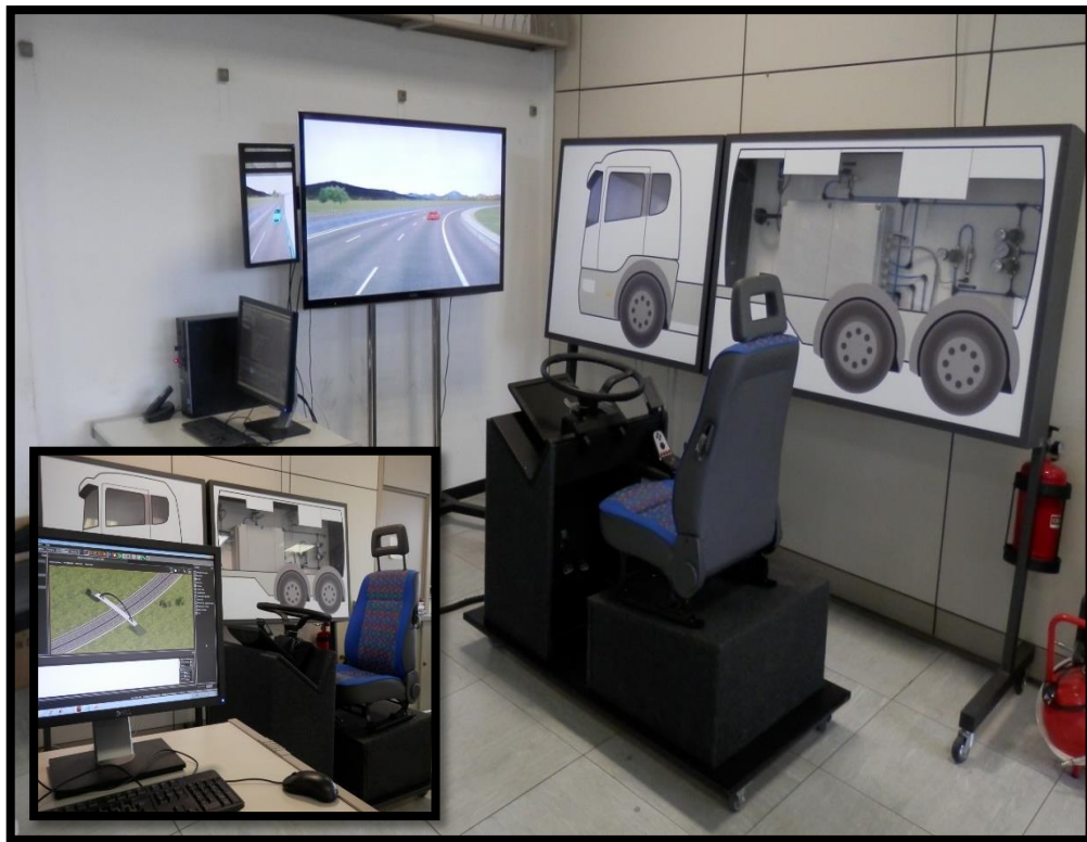
Fig. 3-6. The overall of the 3D driving simulator setup: SCANeR, Simulator server, Controllers, Screen
