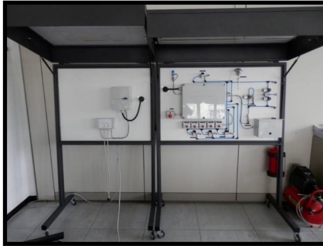
Fig. 3-3. Synoptic panel, a replica of the on-board unit installed in the trucks
